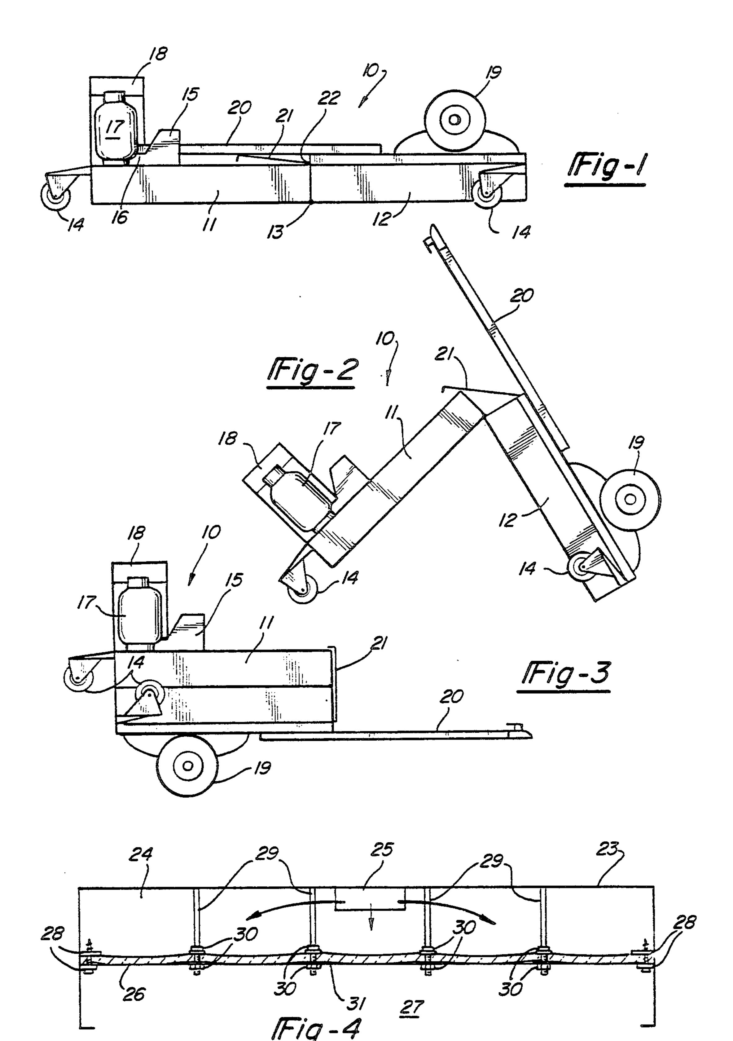
asphalt heater 10 allow manual positioning over the desired areas of pavement.
