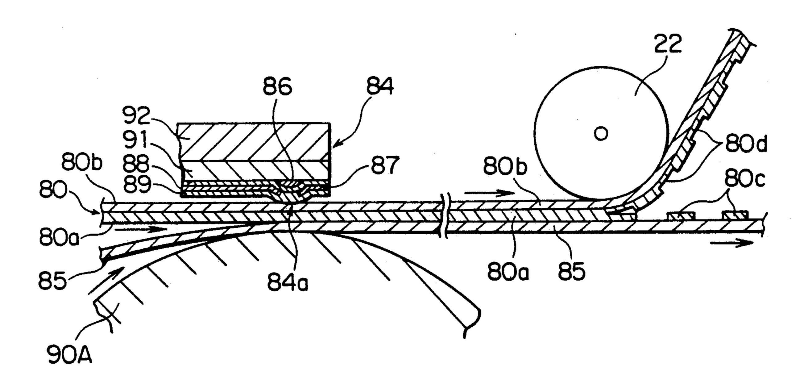
THERMAL TRANSFER RECORDING APPARATUS FOR CONTROLLING PRINTING DENSITY WITH THE TEMPERATURE AT THE POSITION WHERE THE INK RIBBON AND PAPER ARE SEPARATED
