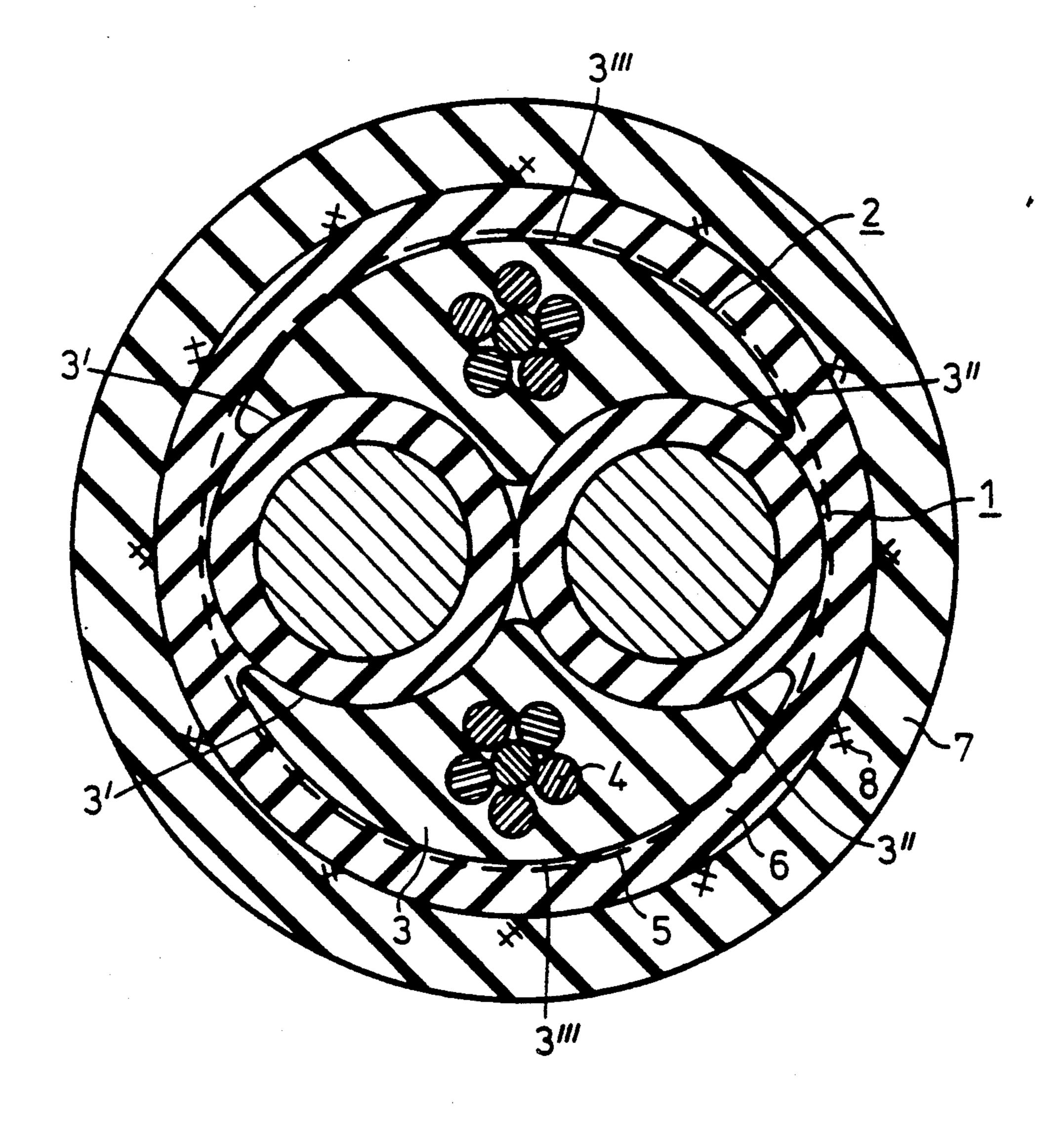
FLEXIBLE ELECTRICAL CABLE HAVING TWO STRANDED CONDUCTORS
