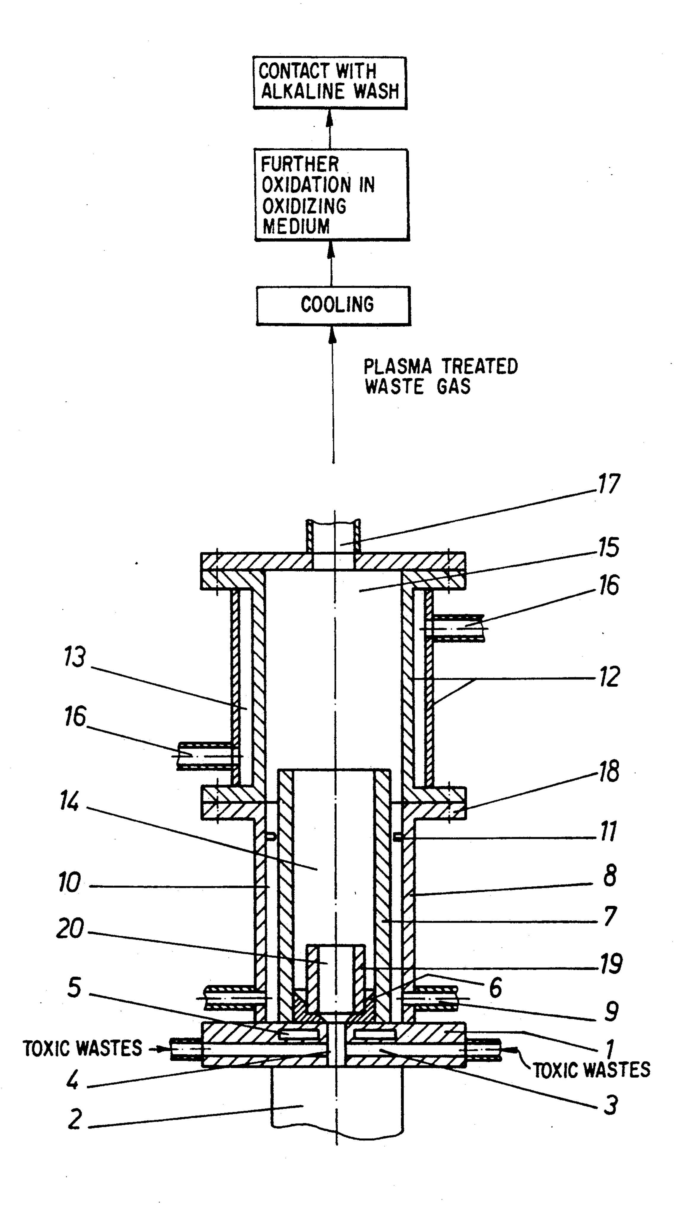
METHOD FOR THE DESTRUCTION OF TOXIC WASTE PRODUCTS AND A PLASMA CHEMICAL REACTOR
