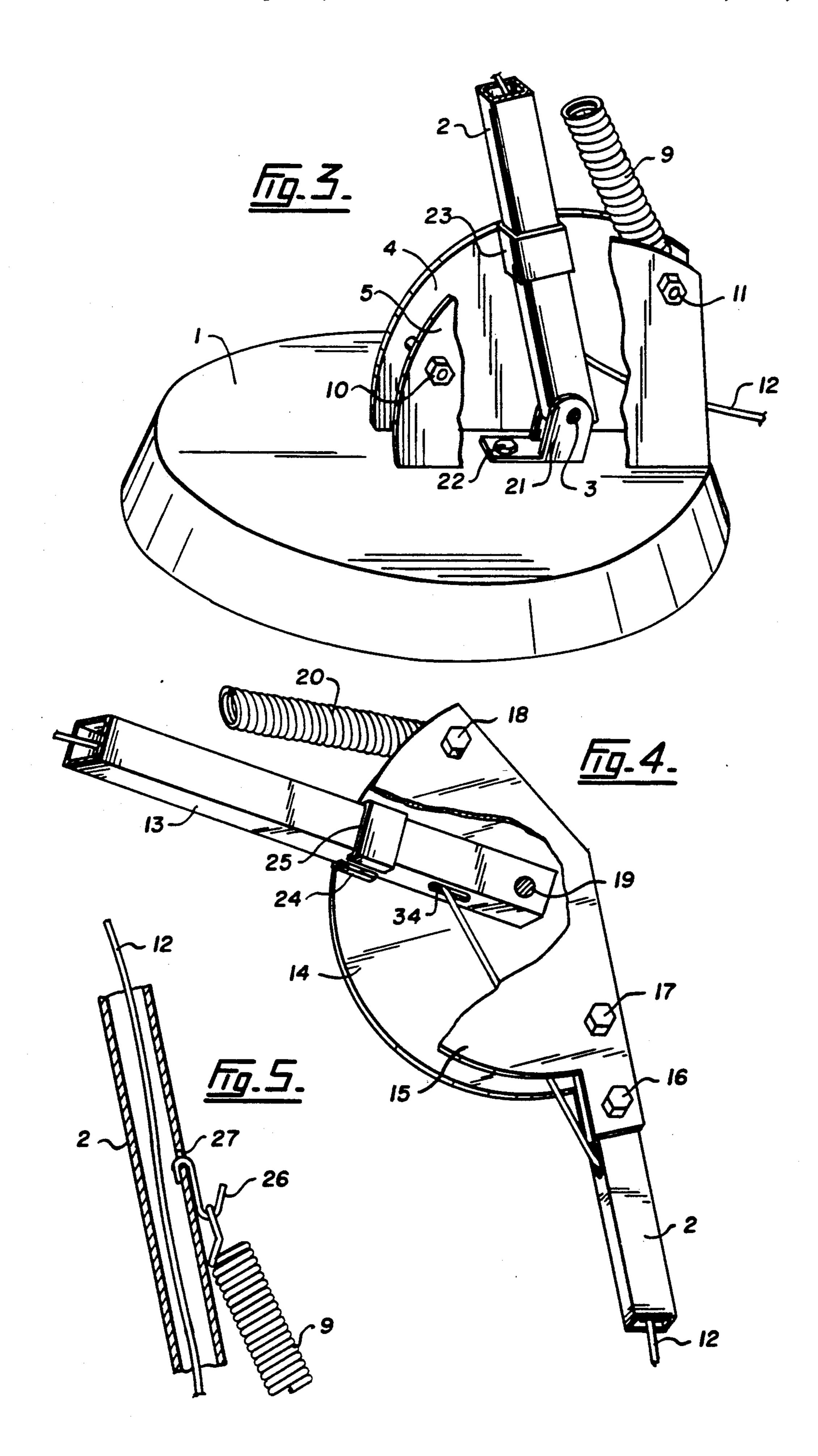
In a second embodiment, a second counterbalanced arm supporting a lamp housing is pivotally attached atop a first counterbalanced arm creating a lamp with a wide variety of adjustable positions.
