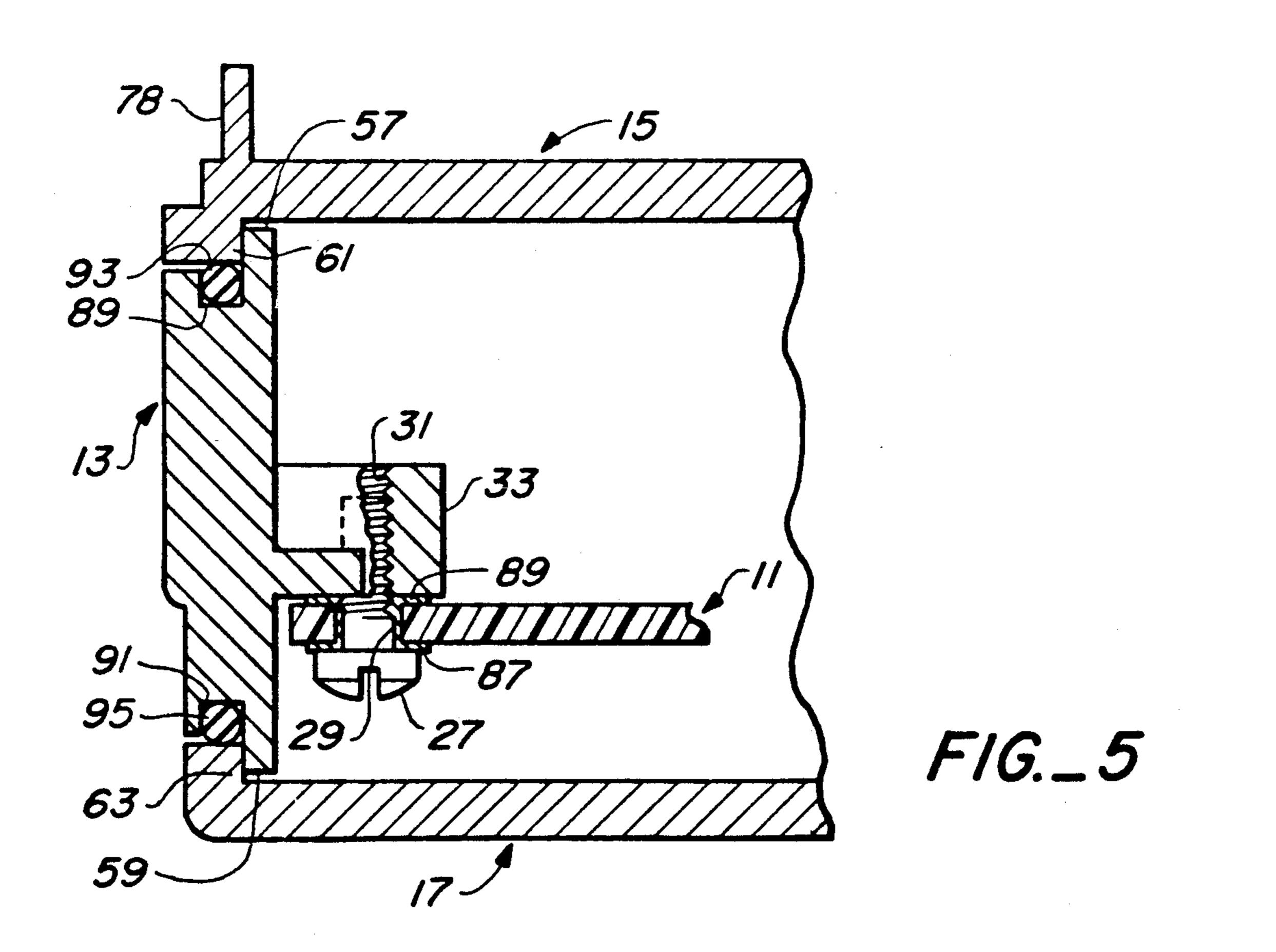
circuit board assembly having a design which facilitates weatherproofing of the printed circuit board and electronic components without introducing a high degree of complexity in accomplishing the sealing.
