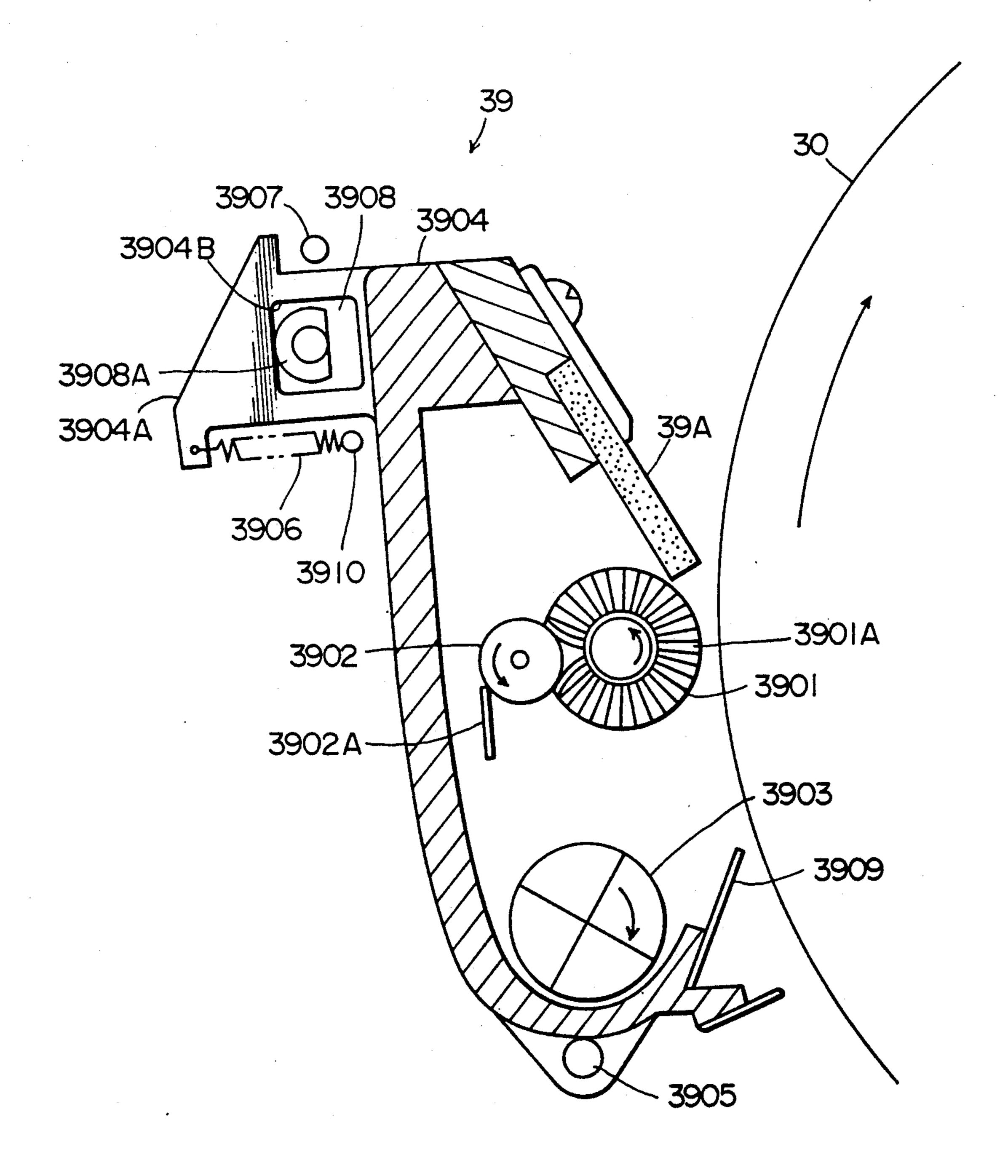
REMOVABLE CARTRIDGE FOR A COLOR IMAGE FORMING APPARATUS
