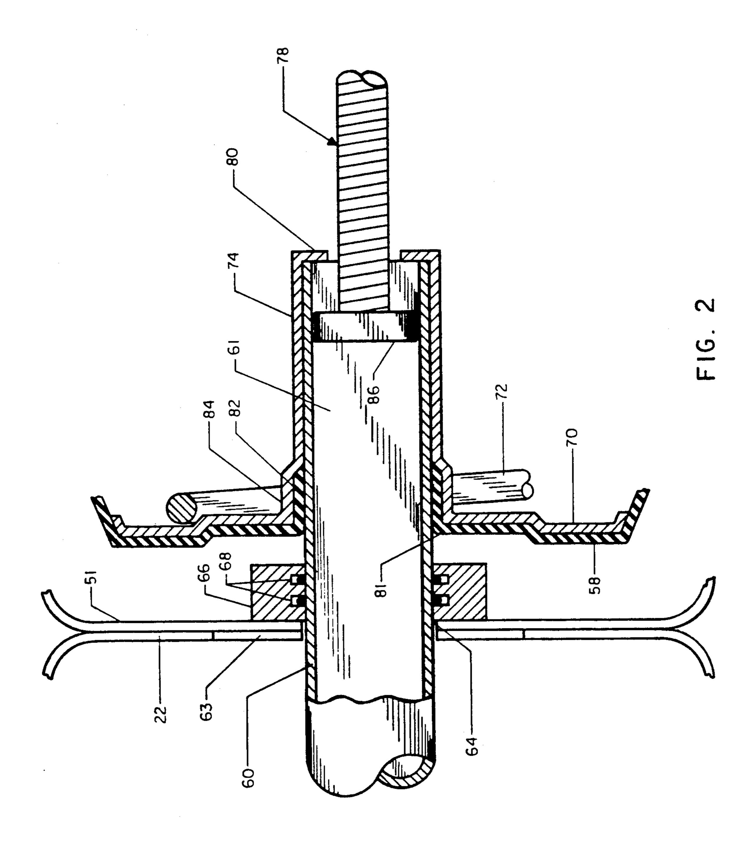
SPRING BRAKE ACTUATOR WITH AN ANNULAR EDGE OF A DIAPHRAGM SEALED BETWEEN A TUBULAR PART OF A PRESSURE PLATE AND AN ACTUATOR ROD
