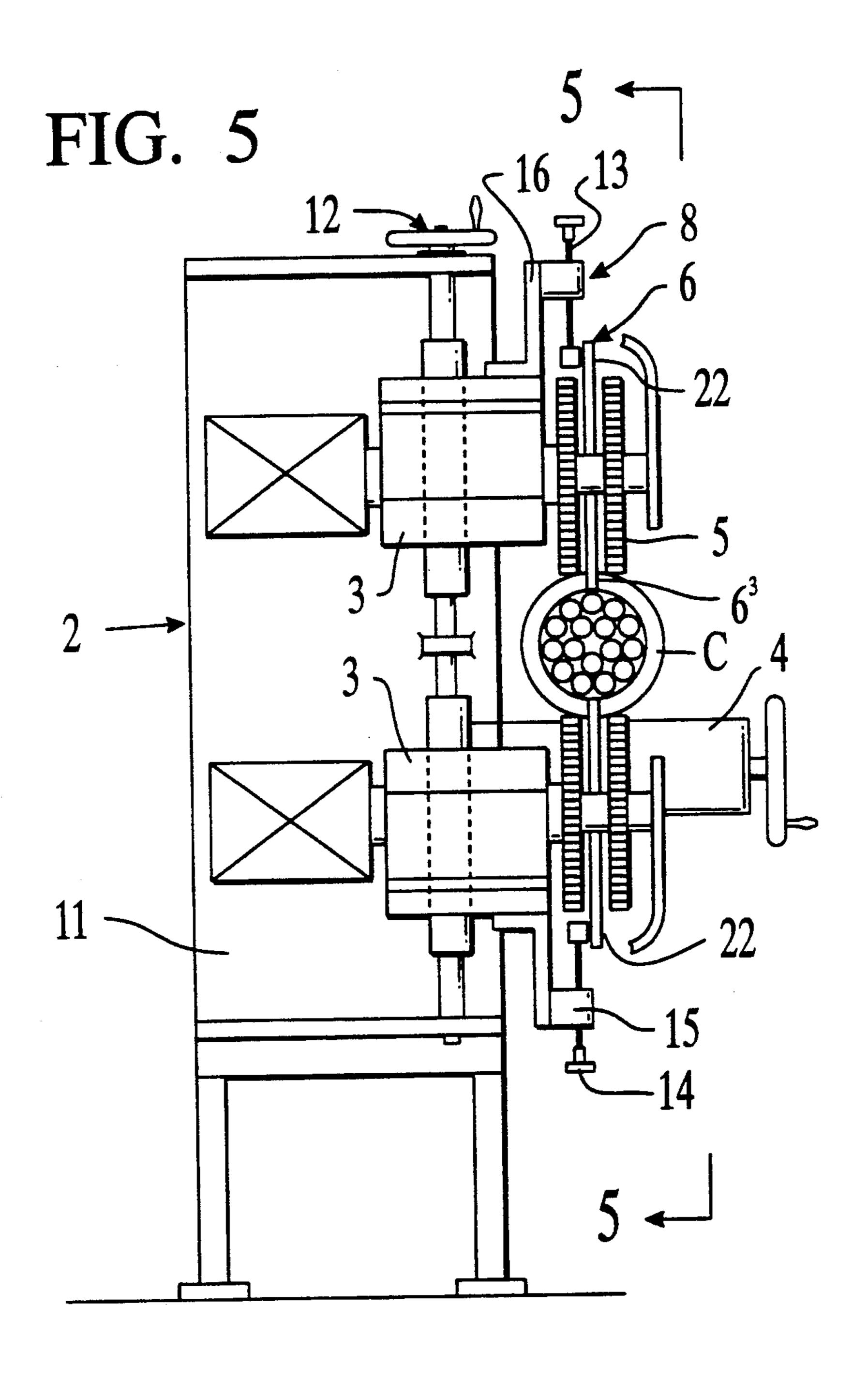
CUTTING DEVICE FOR THE CABLE STRIPPING MACHINES, MORE PARTICULARLY FOR THE PURPOSE OF A RECOVERY OF THESE CABLES
