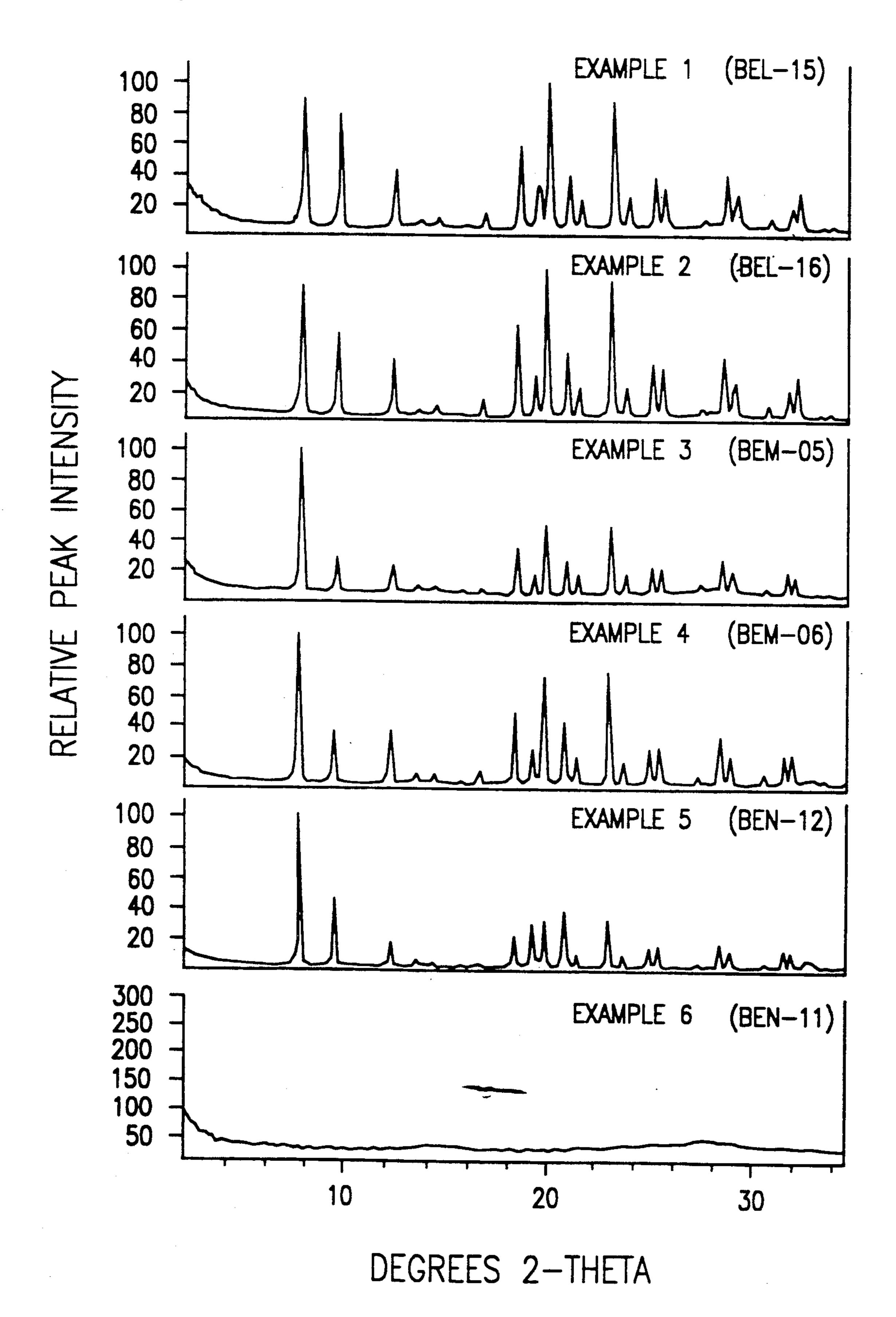
FIG. 2 XRAY DIFFRACTION PATTERNS
