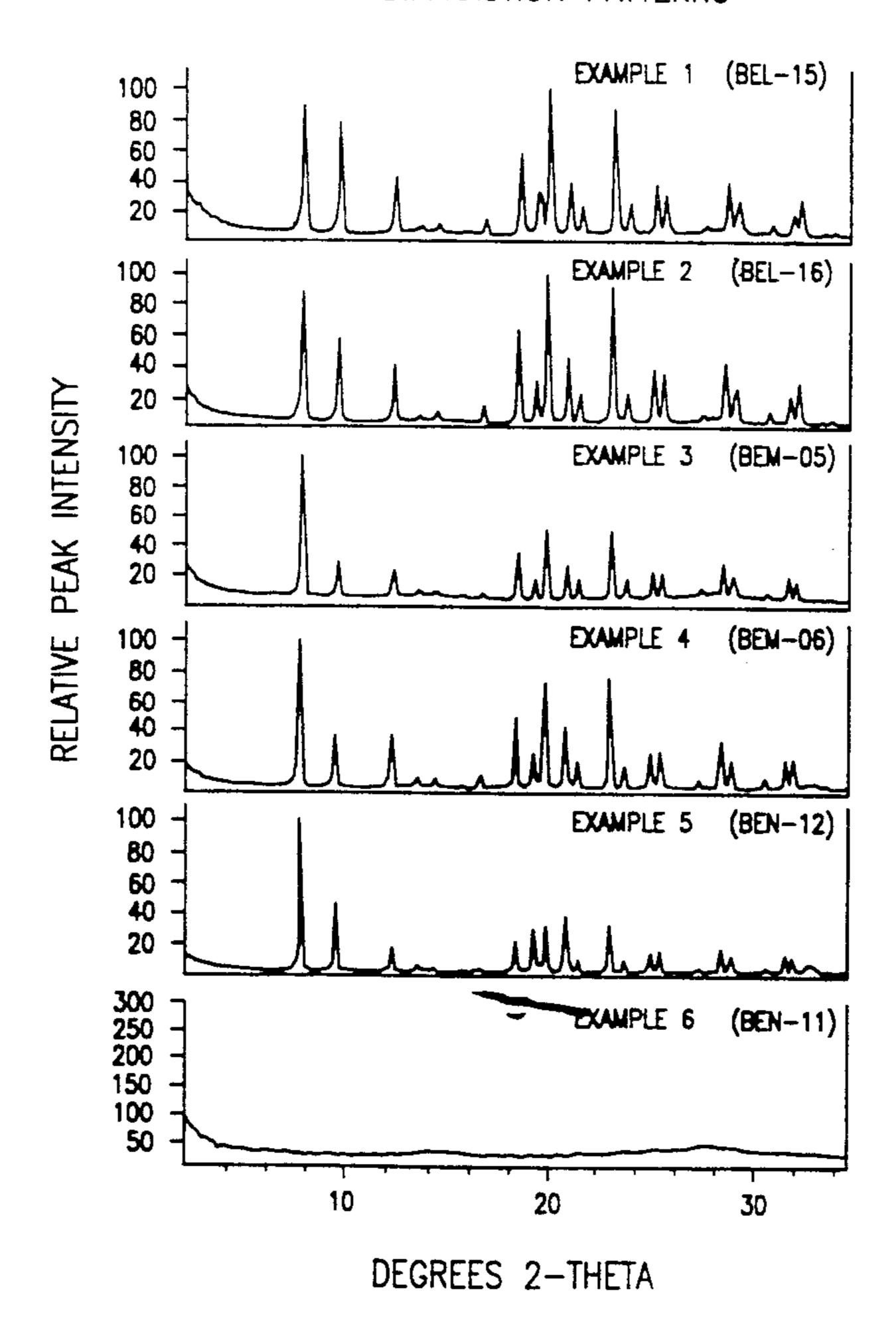
FIG. 1 XRAY DIFFRACTION PATTERNS
