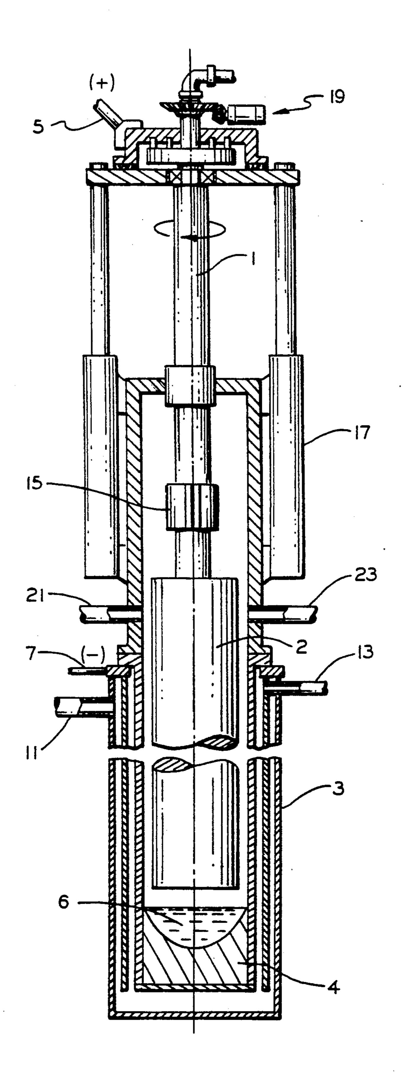
tion taken in connection with the accompanying drawing in which the single FIGURE is a diagrammatic view of an arc furnace incorporating a principal embodiment of the present invention.
