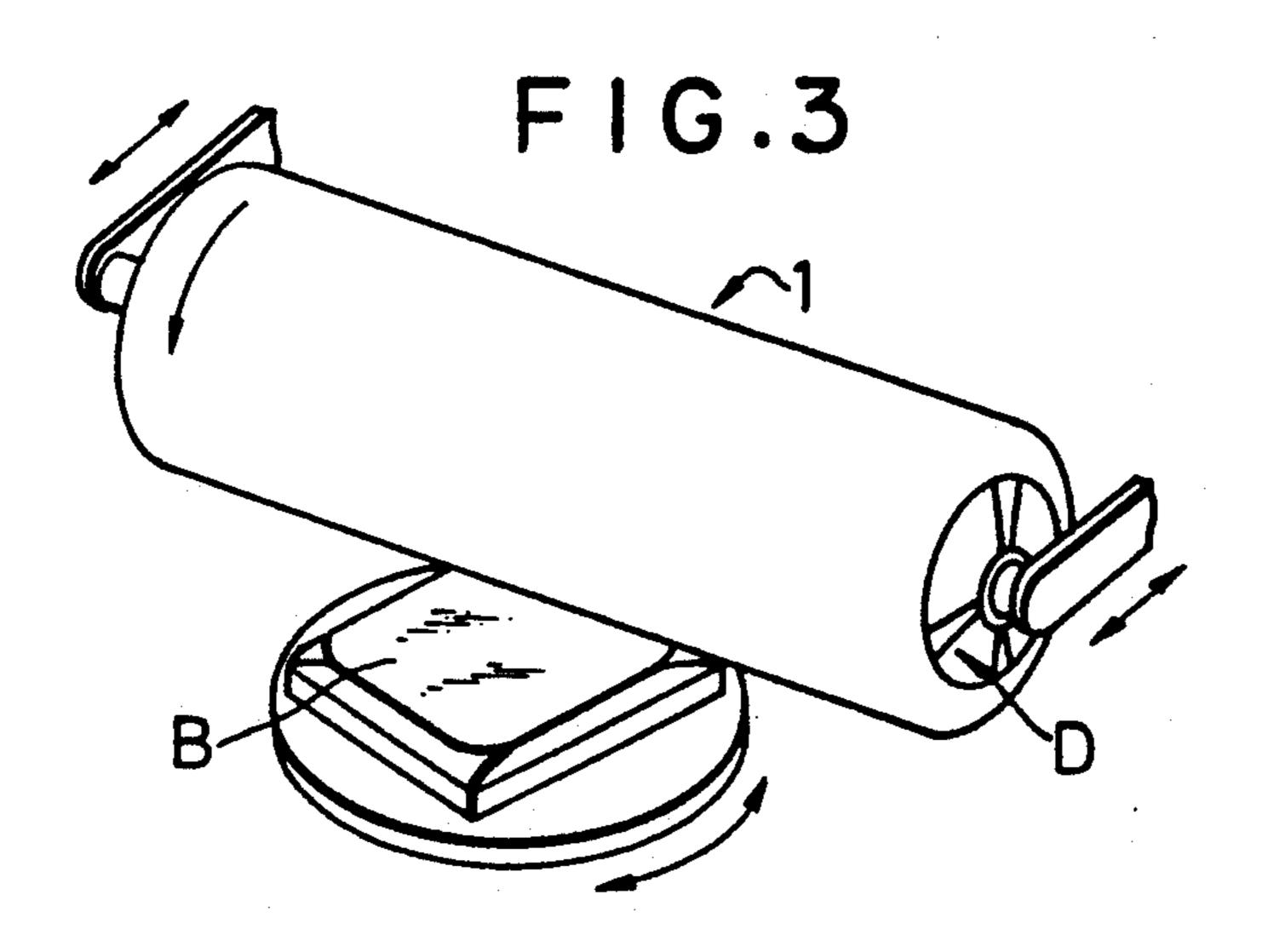
FIG. 3 is a perspective view illustrating how a panel face of a cathode ray tube is ground utilizing a tubular felt.
