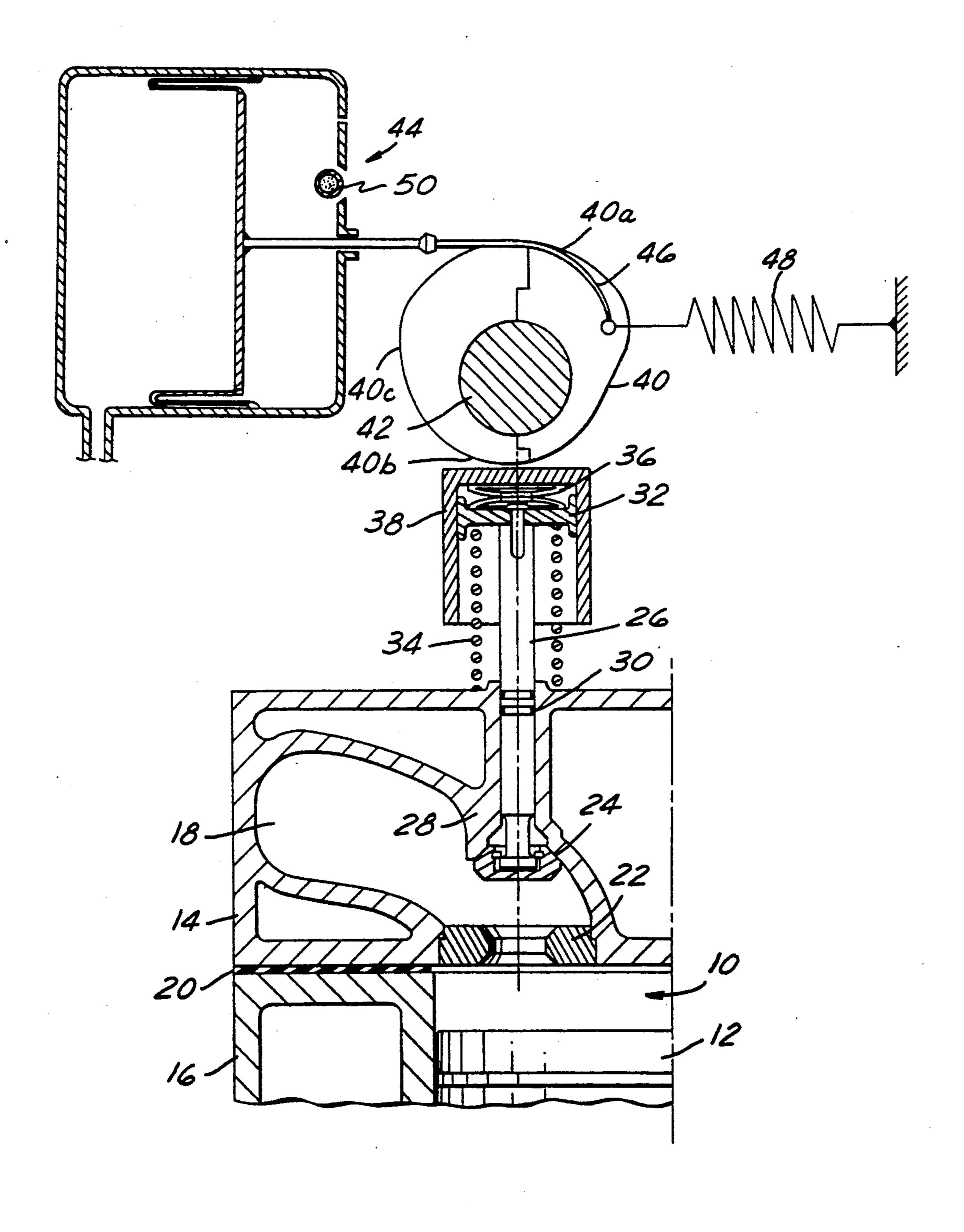
thermore deposits in this gap around the rotor eventually interfere with its operation.
