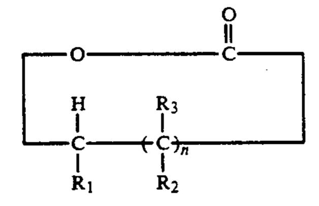
wherein each of R<sub>1</sub>, R<sub>2</sub> and R<sub>3</sub> is H or a C<sub>1</sub>-C<sub>8</sub> alkyl group, and n is an integer of from 1 to 5.
