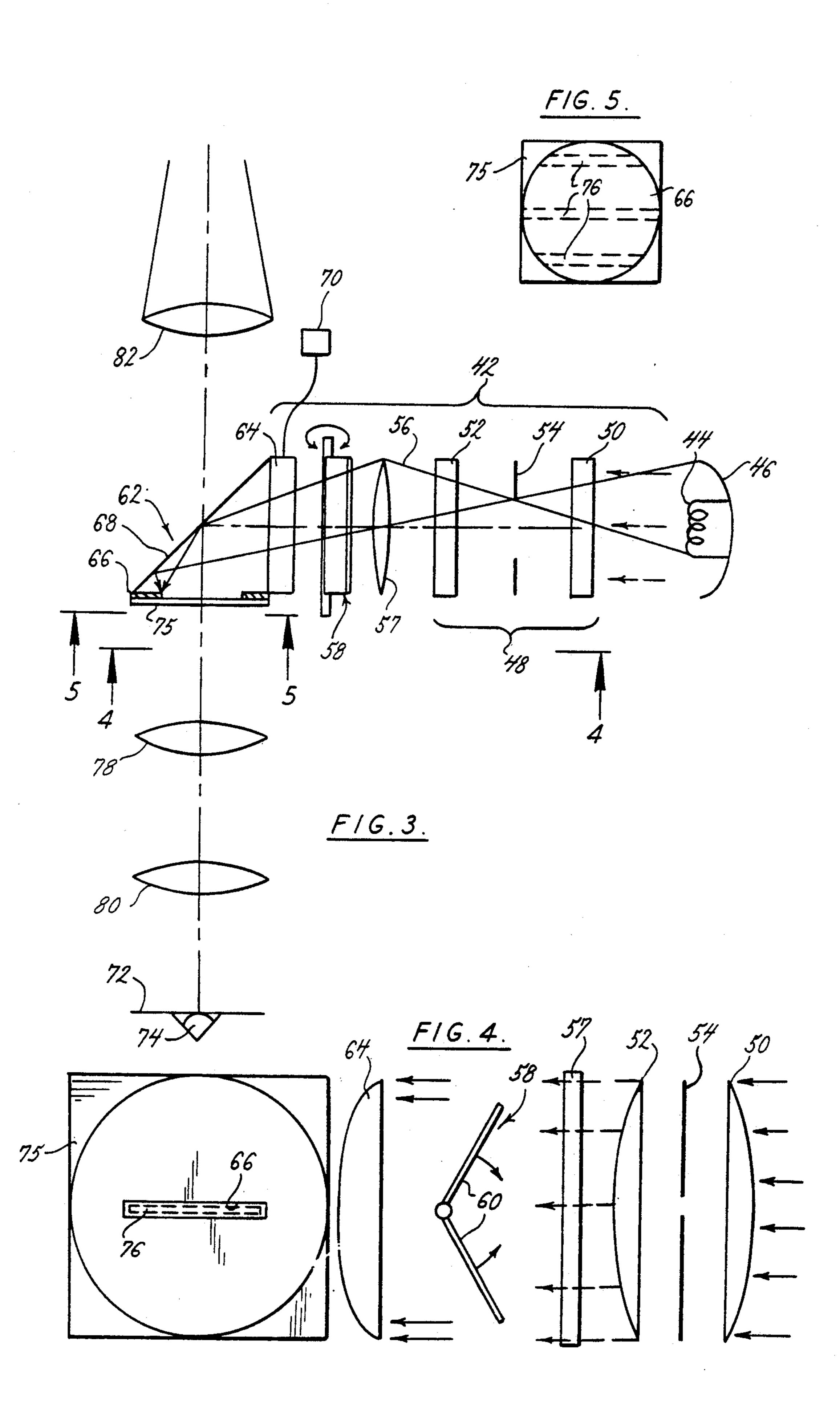
KIT FOR CONVERTING A SLIT LAMP BIOMICROSCOPE INTO A SINGLE APERTURE CONFOCAL SCANNING BIOMICROSCOPE
