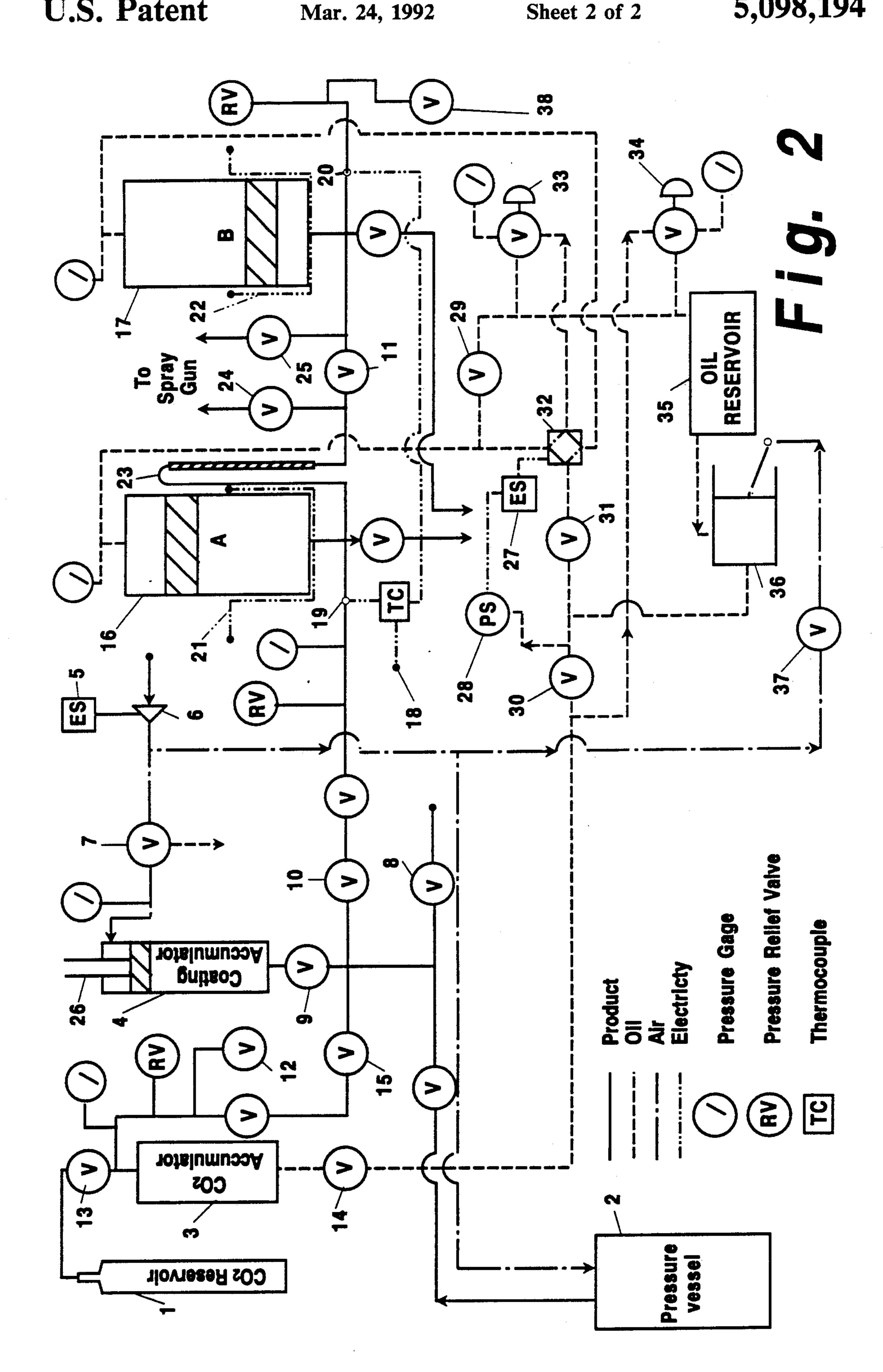
SEMI-CONTINUOUS METHOD AND APPARATUS FOR FORMING A HEATED AND PRESSURIZED MIXTURE OF FLUIDS IN A PREDETERMINED PROPORTION
