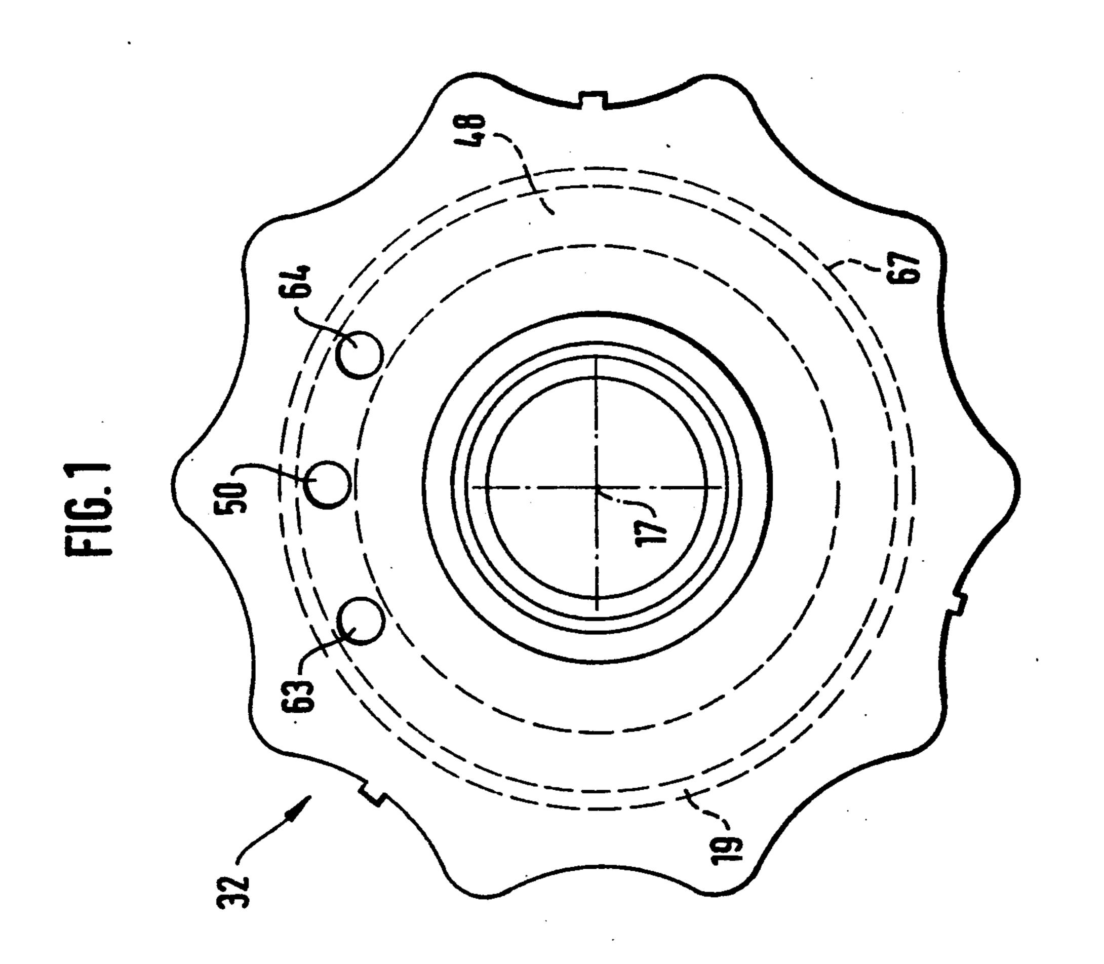
together, thus weakening the cap and possibly producing a predetermined breaking point. Furthermore, the through airholes are then sufficiently far apart so that something that causes the blockage of one of the through airholes does not also affect the other.
