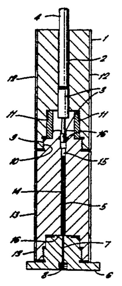
to have a melting point of at least 139.5° C. and a density of at least 0.98 g/cm<sup>3</sup>. Thereafter the workpiece of polyethylene is deformed in the solid phase to provide a polyethylene product by, for example, passage through a die, the workpiece being subjected to a deformation extrusion ratio of at least 3 and preferably 3 to 25. The process in accordance with the invention allows more
