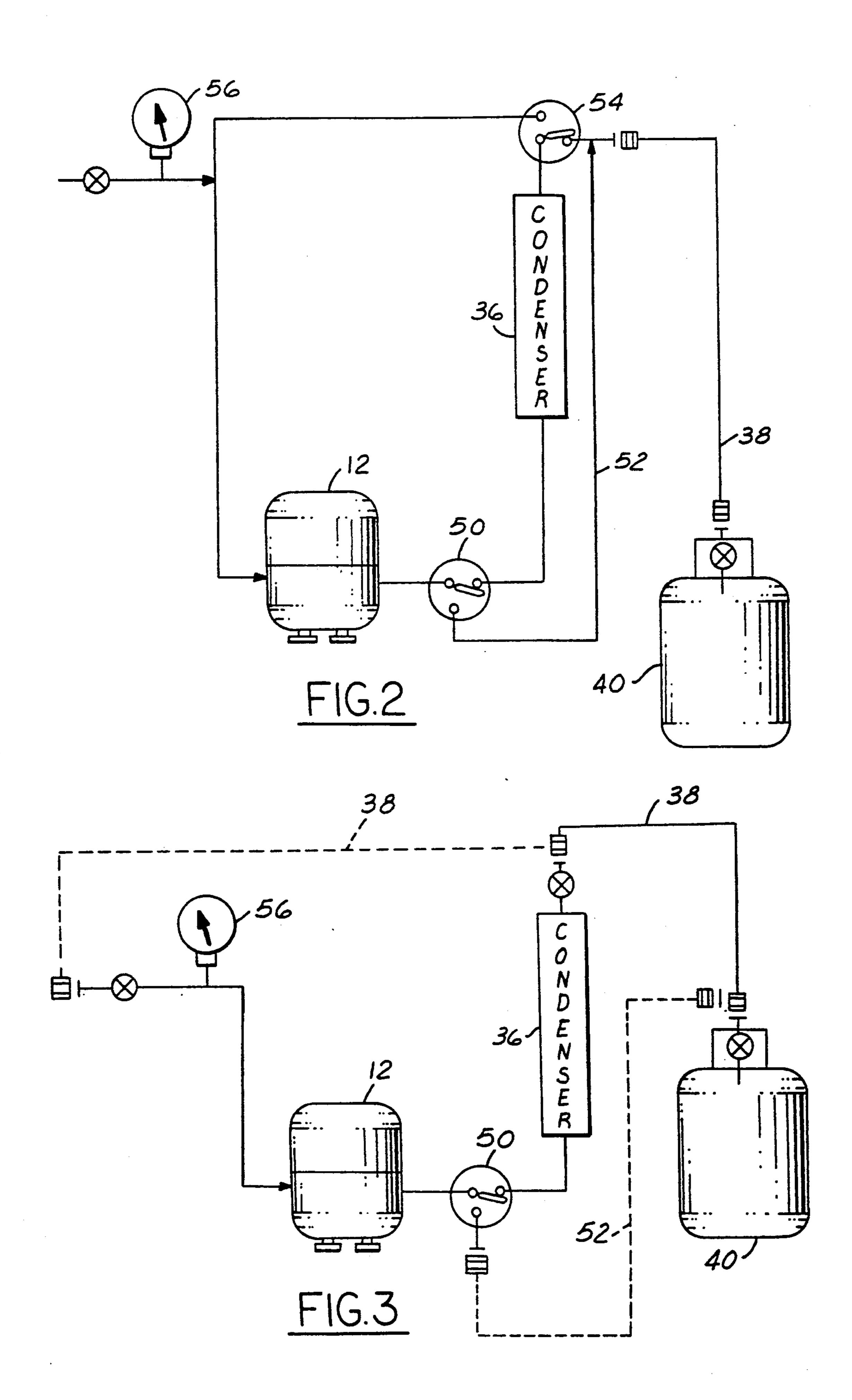
REFRIGERANT HANDLING SYSTEM AND METHOD WITH MULTIPLE REFRIGERANT CAPABILITY
