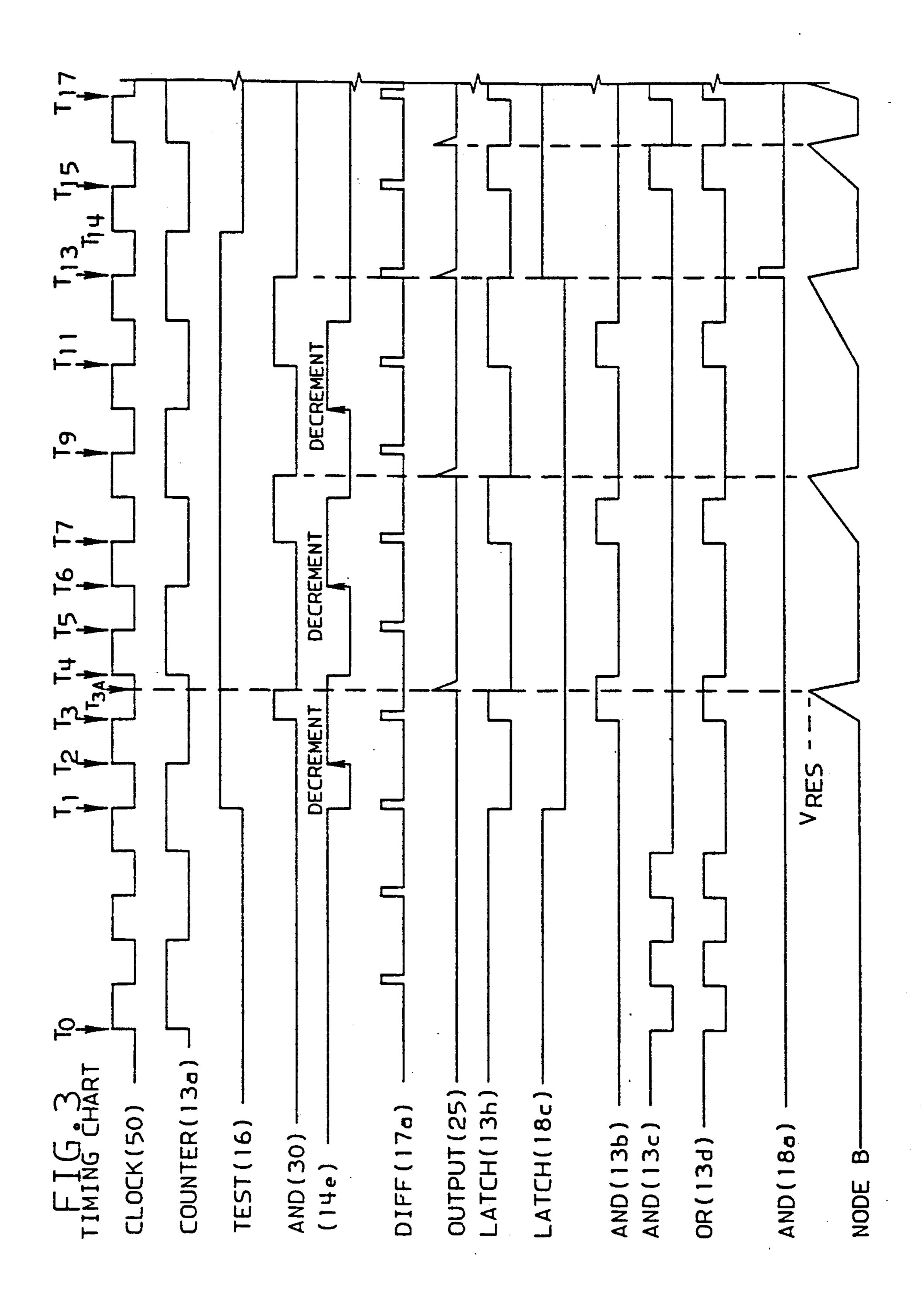
The present invention is thus a circuit, for generating timing edges within a clock cycle which timing edges can be any function of the clock cycle.
