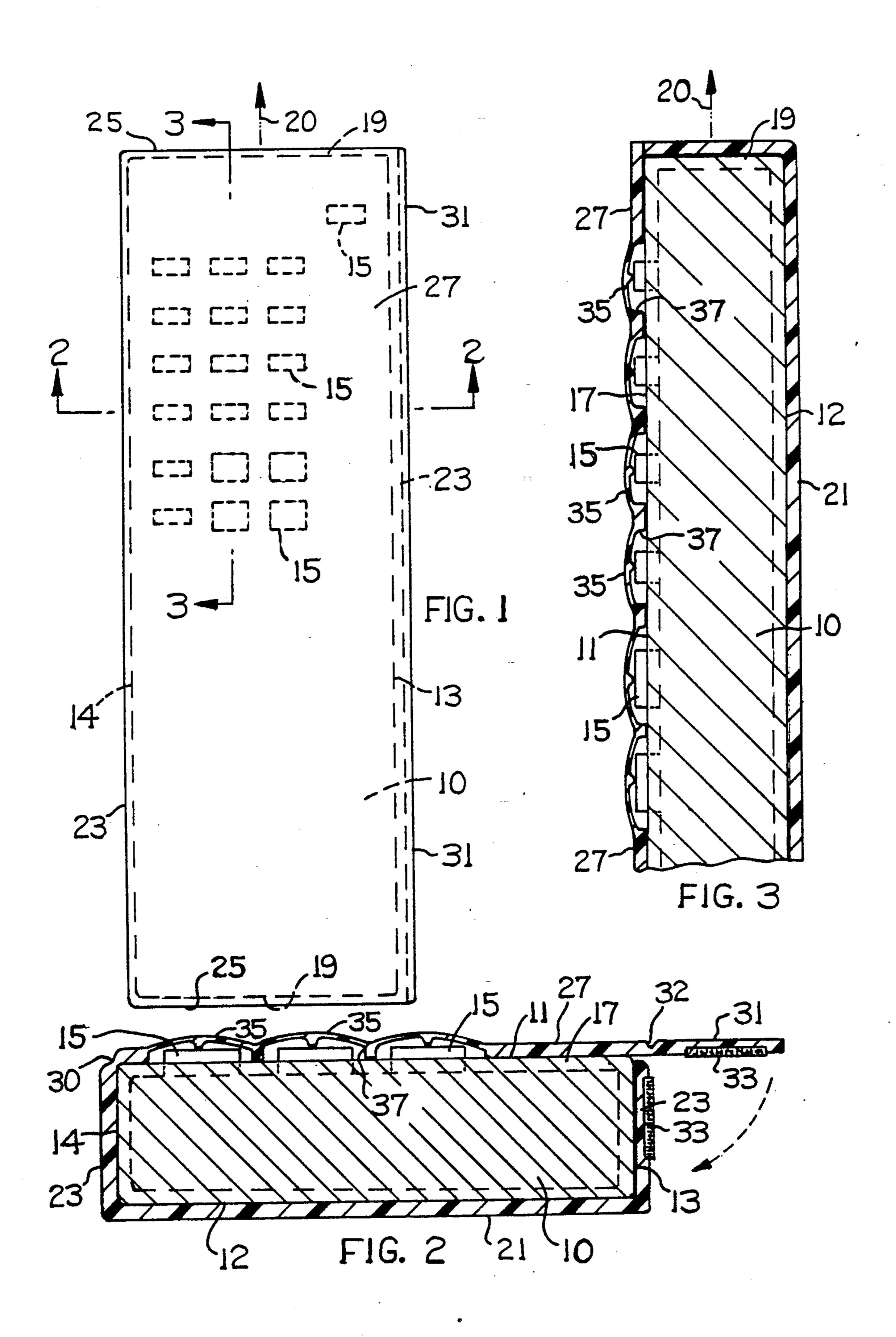
mine a desired pushbutton location simply by running the thumb or first finger across the upper face of the control unit. Each pushbutton is operated by depressing the button downwardly about one half its projected
