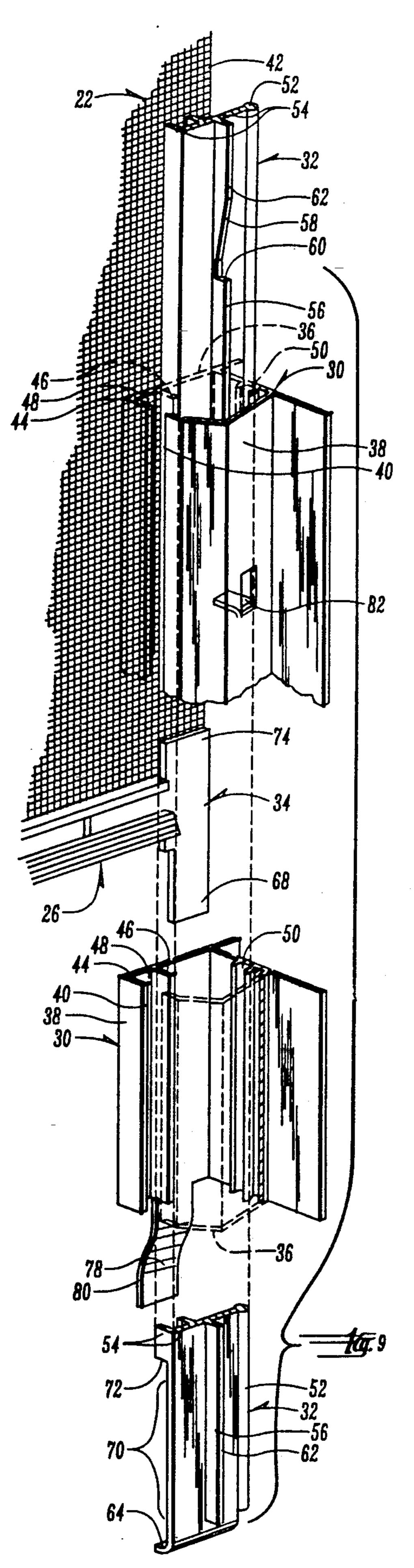
gagement with the guide channel actuation tab when the screen is in its lowered position.
