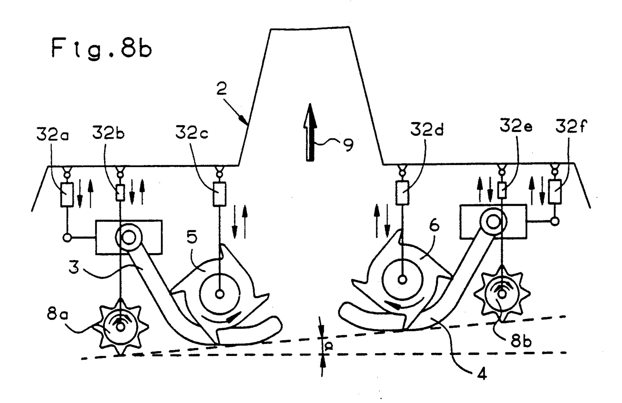
BALE OPENING METHOD AND DEVICE HAVING ROLLERS AND GRATE BARS ADJUSTABLE IN HEIGHT RELATIVE TO ONE ANOTHER, FOR DETACHING FIBER TUFTS FROM THE TOP SURFACE OF A BALE
