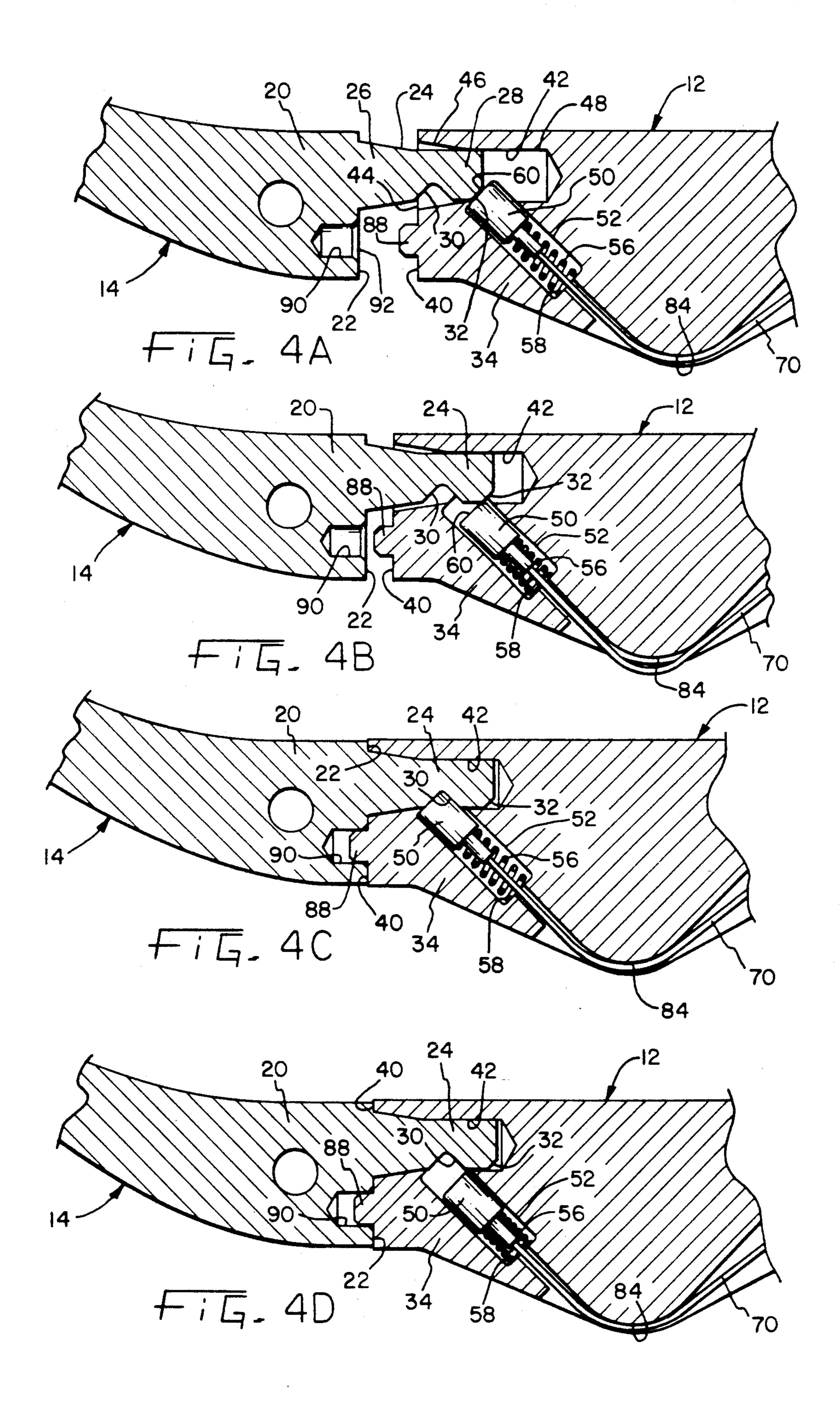
rate disengaging mechanism is operable by the surgeon to permit axial separation of the cutter and handle.
