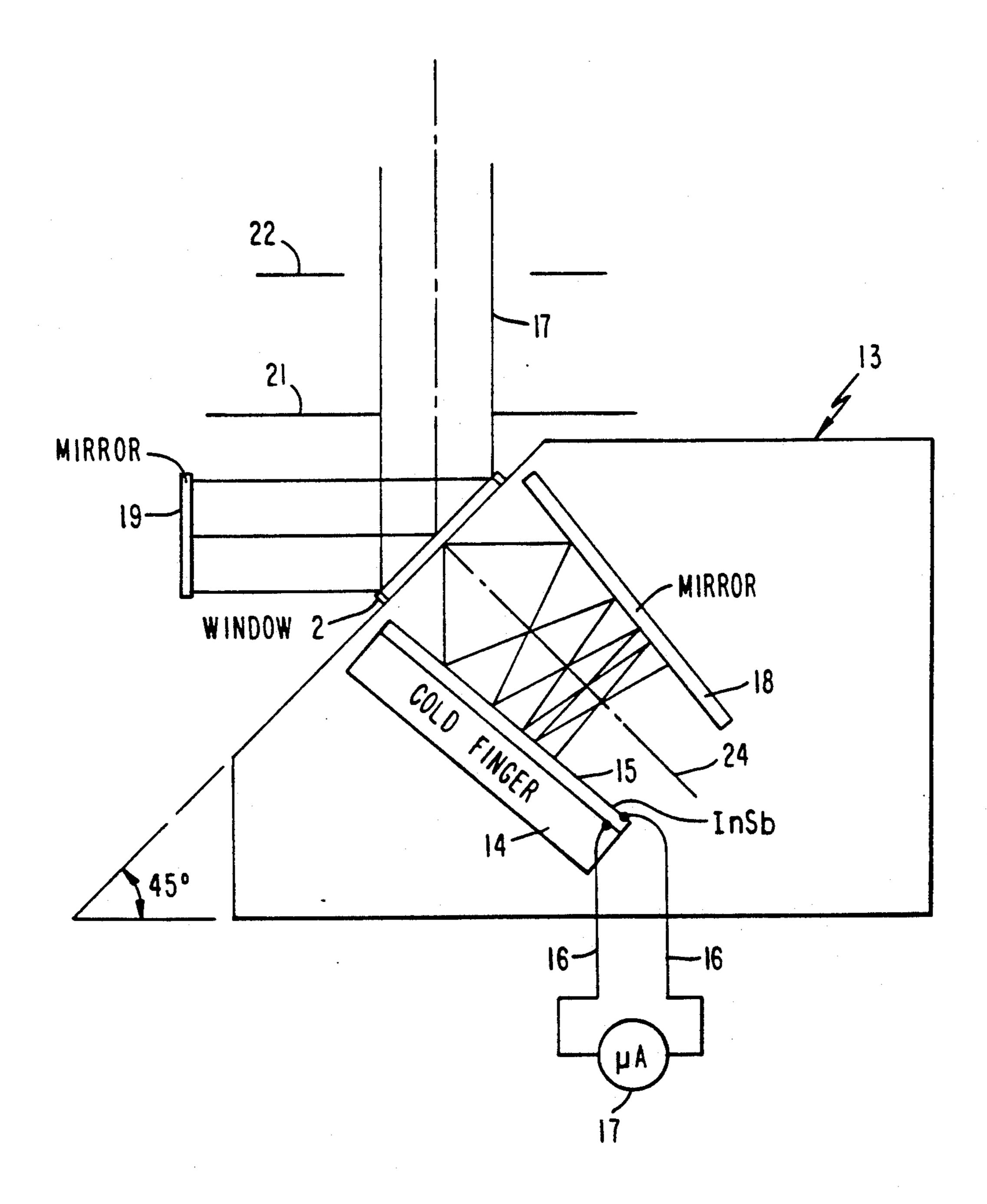
that collects and accurately measures infrared radiation incident on a detector aperture in the band from 2.5 to 5 micrometers.
