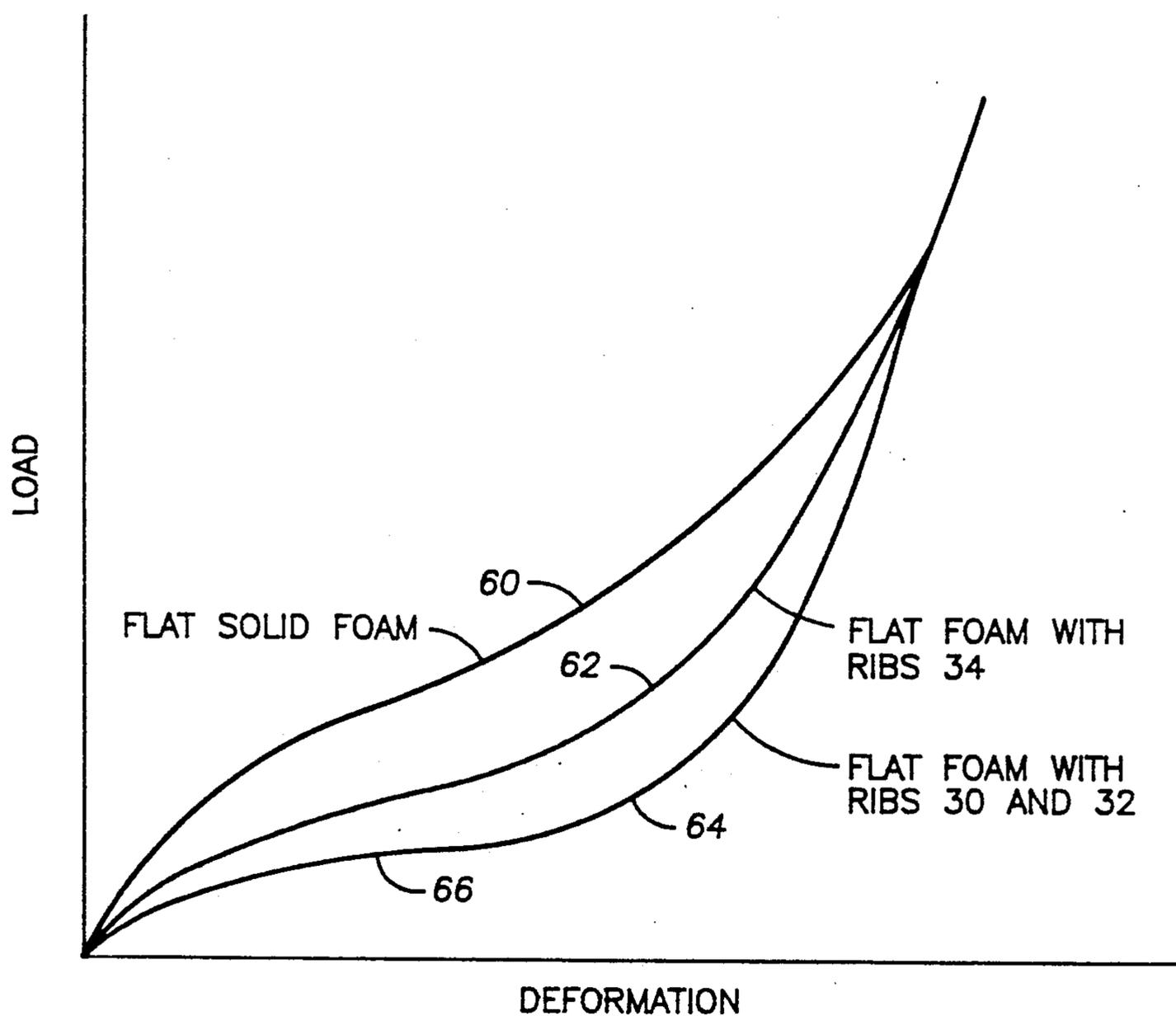
TYPICAL LOAD/DEFORMATION CURVES
