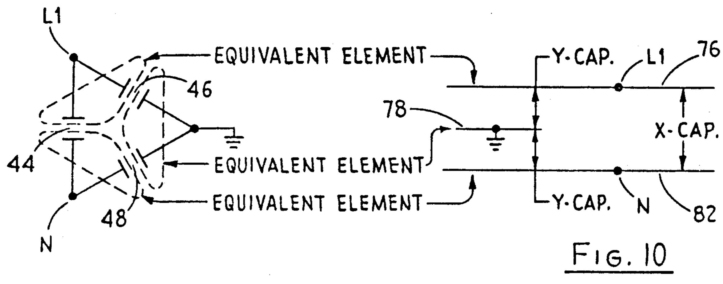
INTEGRATED ELECTROMAGNETIC INTERFERENCE FILTER
