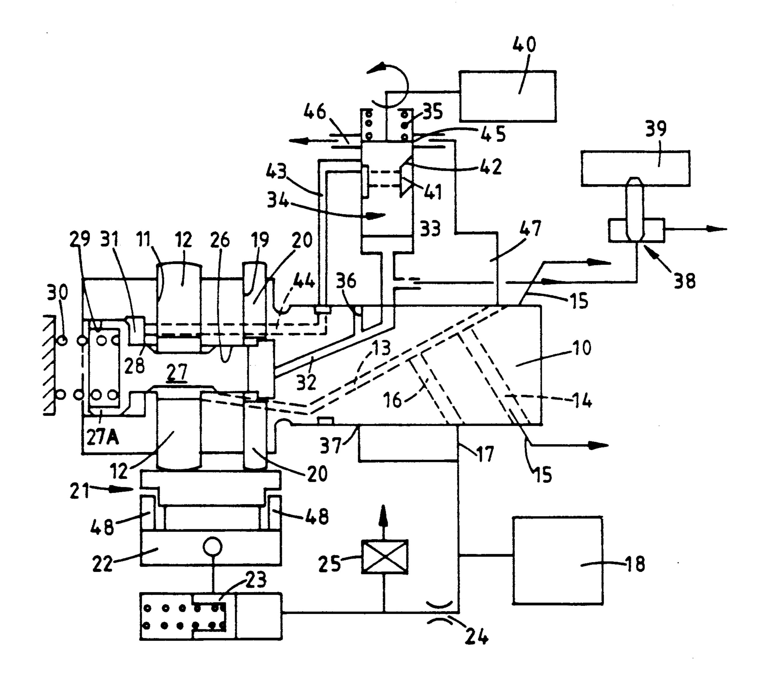
In both forms of the pump as described above, the spill path is constituted by the plungers and very careful construction of the plungers is therefore required. Moreover, the area of the spill path may not be sufficient to ensure the required rate of spillage of fuel.
