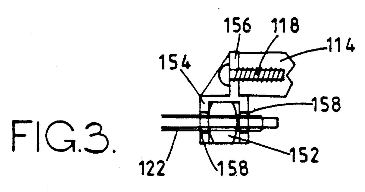
adjustment member and a screw-threaded region associated with the screw-threaded rod.
