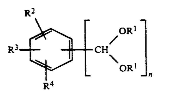
where R<sup>1</sup> is alkyl of 1 to 6 carbon atoms, R<sup>2</sup>, R<sup>3</sup> and R<sup>4</sup> are hydrogen or halogen, straight-chain, branched or cyclic hydrocarbon radicals or alkoxy, acyloxy, aryloxy or aralkoxy, and n is 1 or 2, in which benzyl derivatives of the general formula
