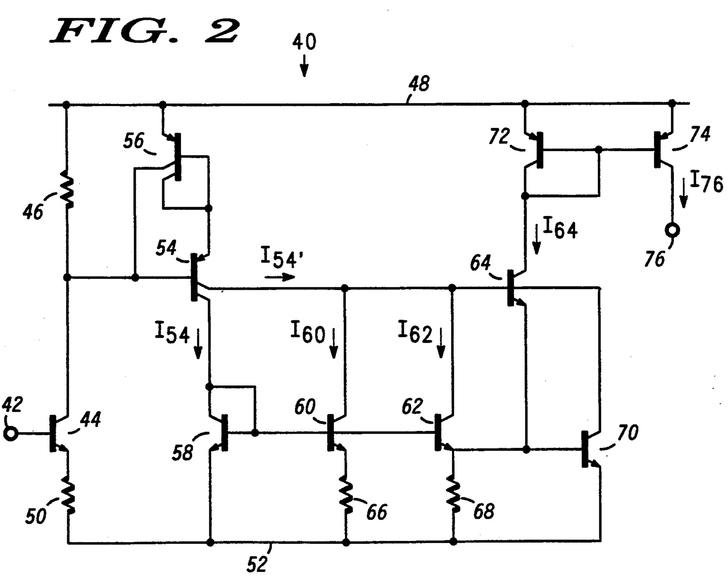
second collector of the first transistor and a collector for providing an output signal when the input signal exceeds a first predetermined threshold. The output signal is substantially zero when the input signal is less
