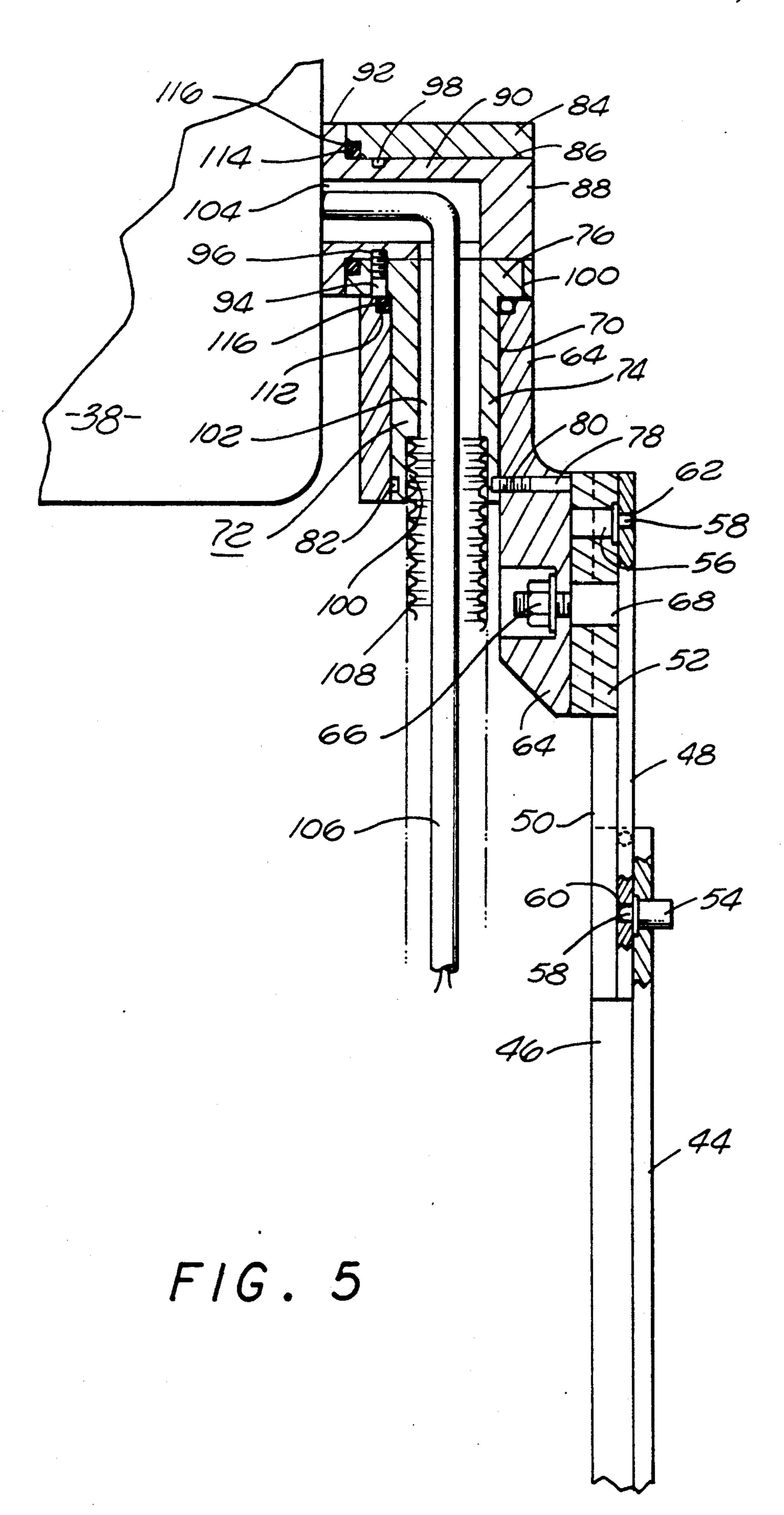
FIG. 5 is a cross-sectional view, showing the "pop-5 up" mechanism of the viewing device.
