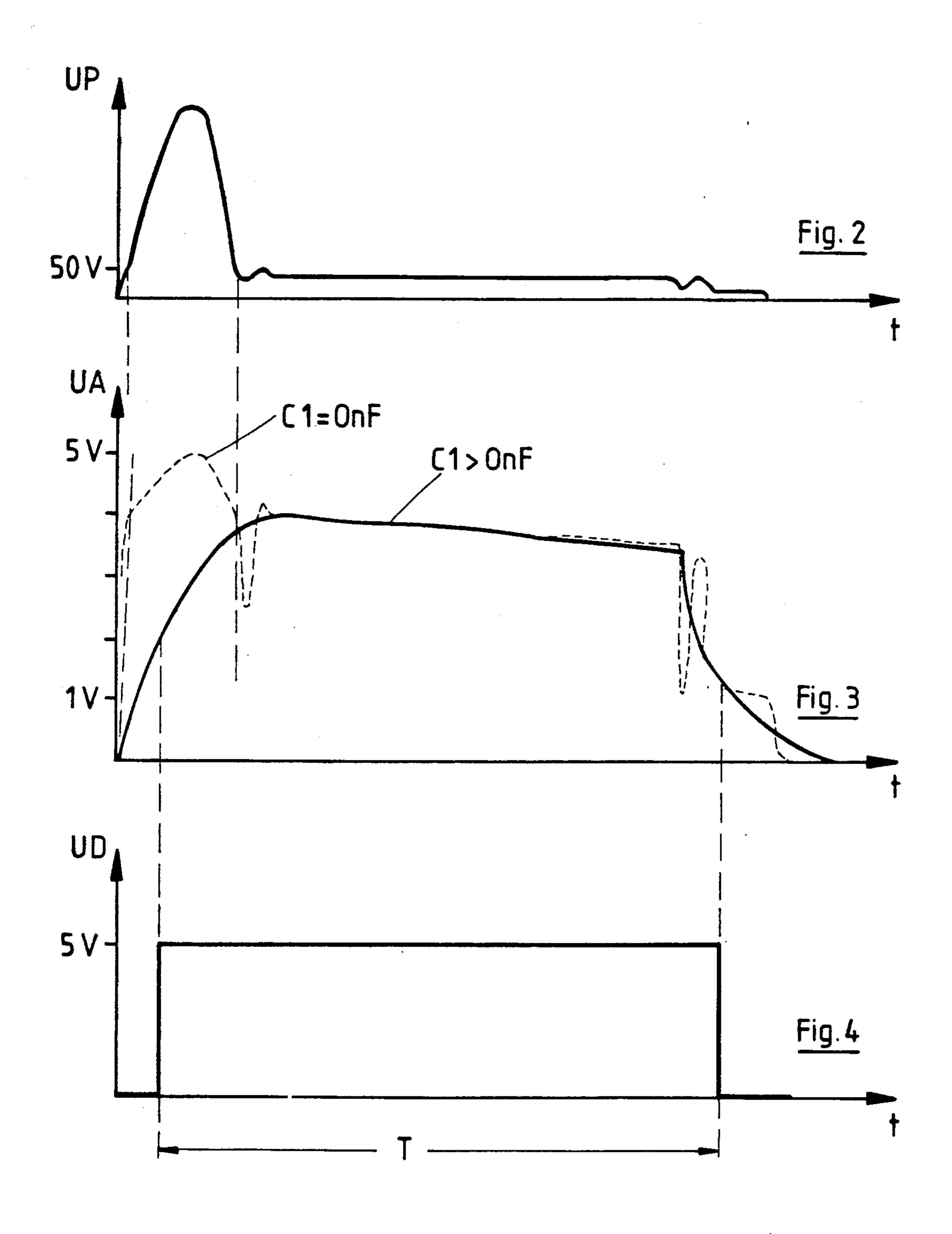
CIRCUIT APPARATUS FOR MEASURING THE PRIMARY VOLTAGE OF AN IGNITION COIL
