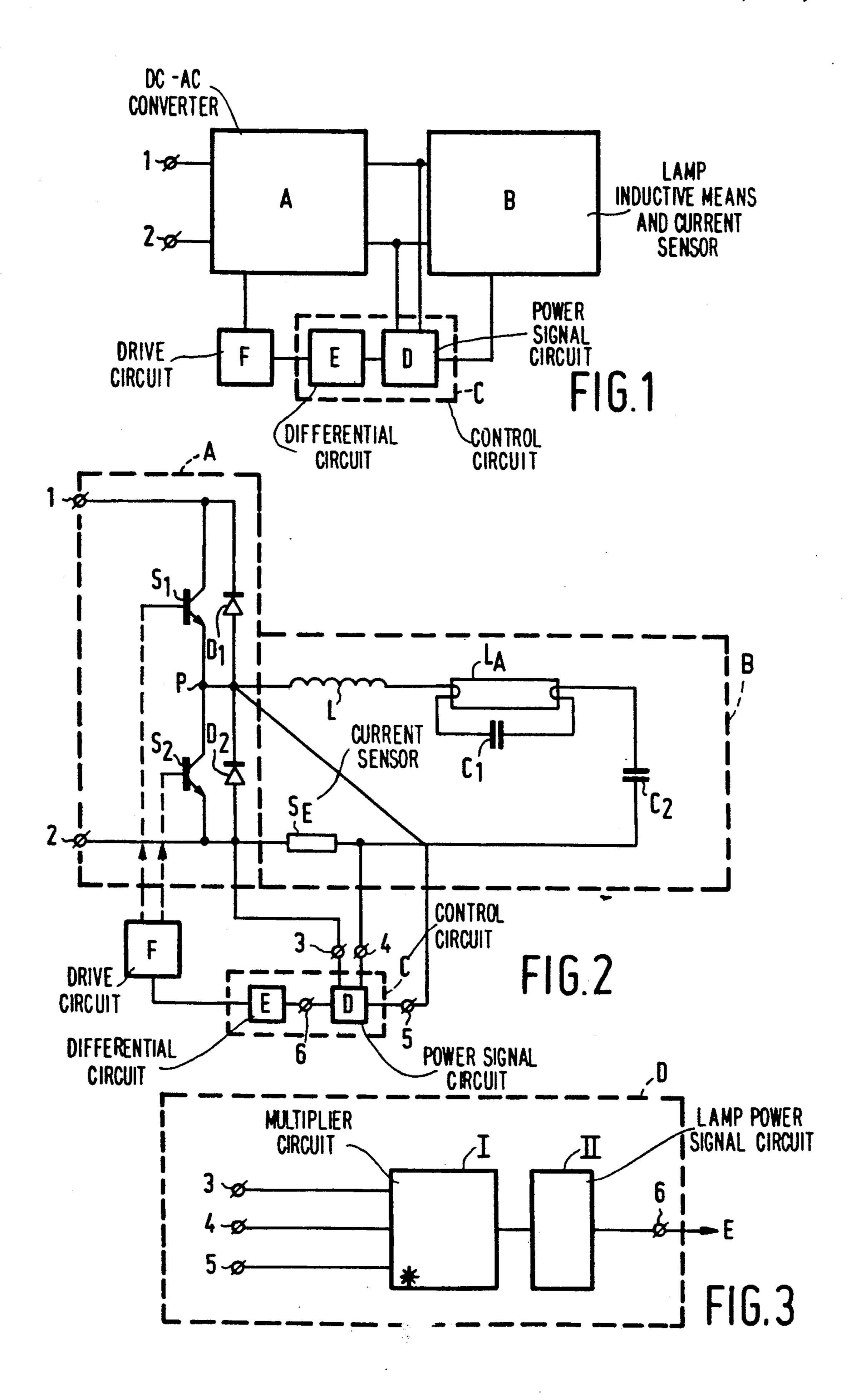
DC-AC converter can be controlled in a simple manner, while this power control is dependent exclusively on the current through the load circuit.
