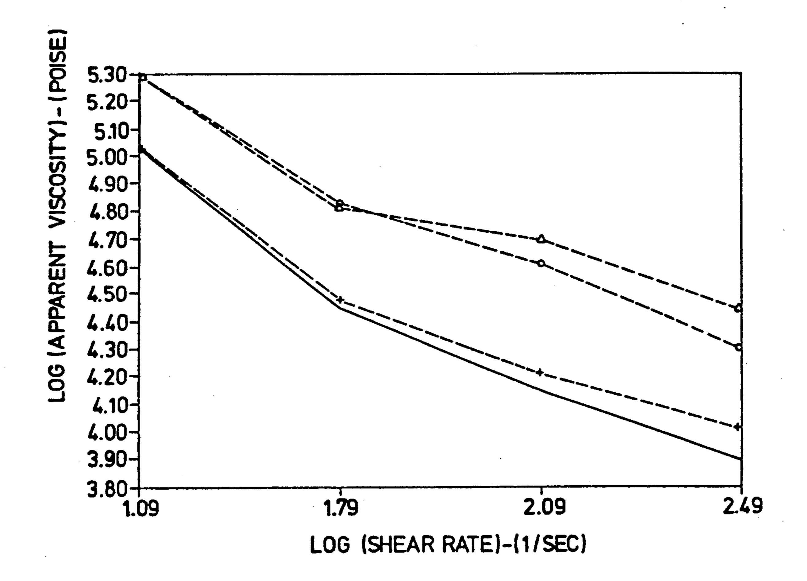
PLOT OF LOG (APPARENT VISCOSITY IN POISE) VERSUS LOG (SHEAR RATE IN 1/SEC). DATA WAS OBTAINED ON A MONSANTO PROCESSABILITY TESTER.
