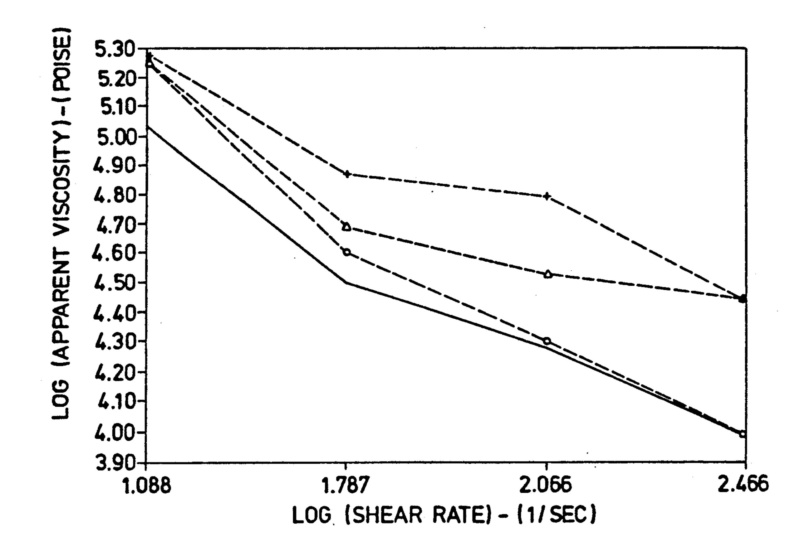
PLOT OF LOG (APPARENT VISCOSITY IN POISE) VERSUS LOG (SHEAR RATE IN 1/SEC). DATA WAS OBTAINED ON A MONSANTO PROCESSABILITY TESTER.
