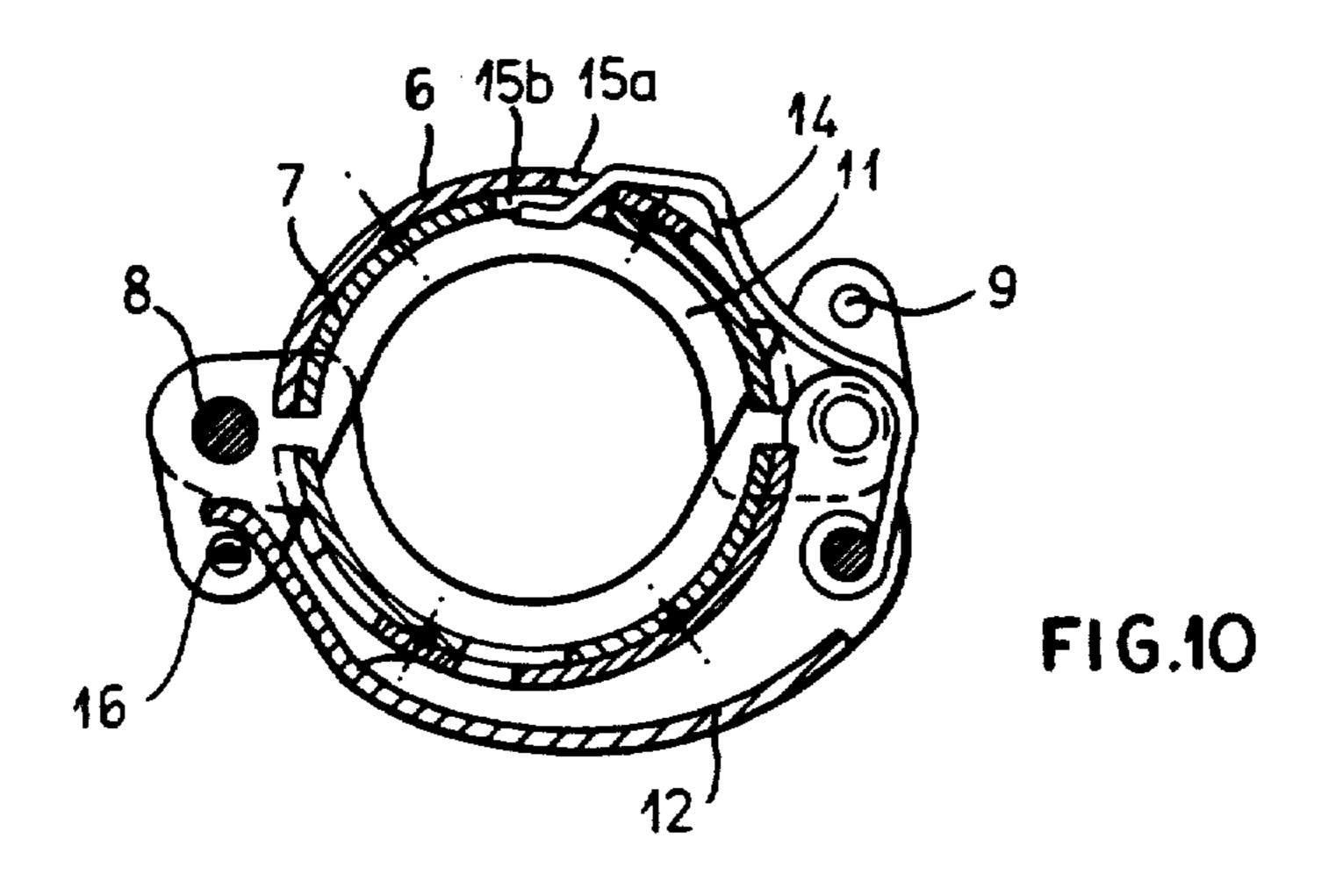
DEVICE FOR CONNECTING THE END OF A HOSE TO A CONNECTING SPIGOT
