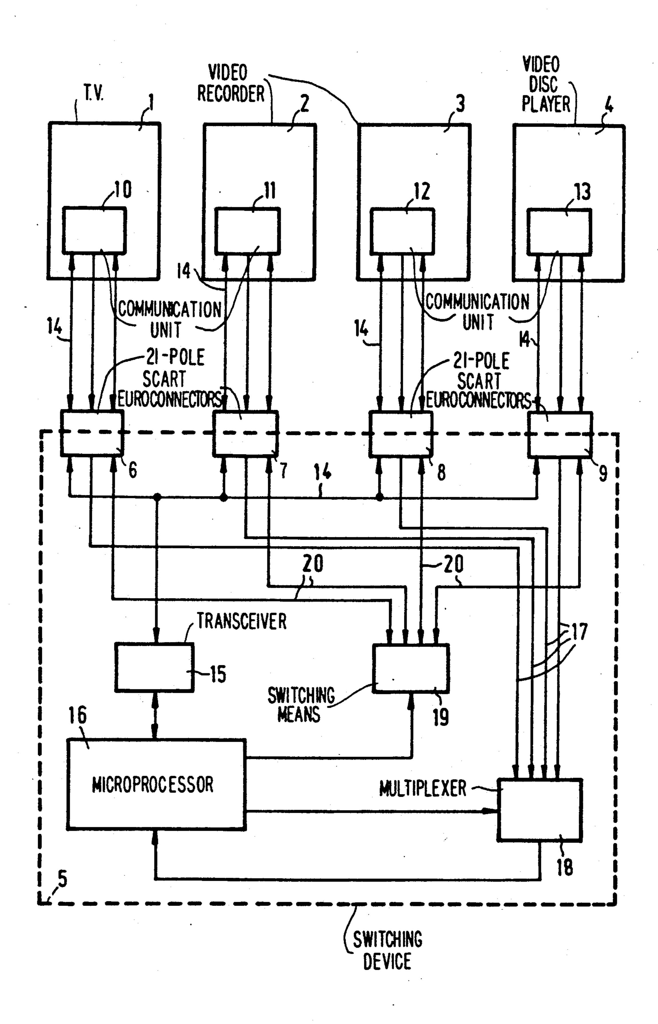
METHOD OF ESTABLISHING A SIGNAL PATH BETWEEN AT LEAST TWO APPARATUSES AND AN ARRANGEMENT OF AT LEAST TWO APPARATUSES FOR REALISING THE METHOD
