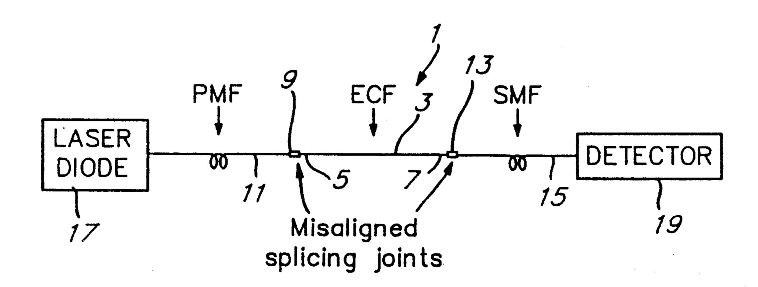
PMF - Single-Mode Polarization Maintaining Fiber
