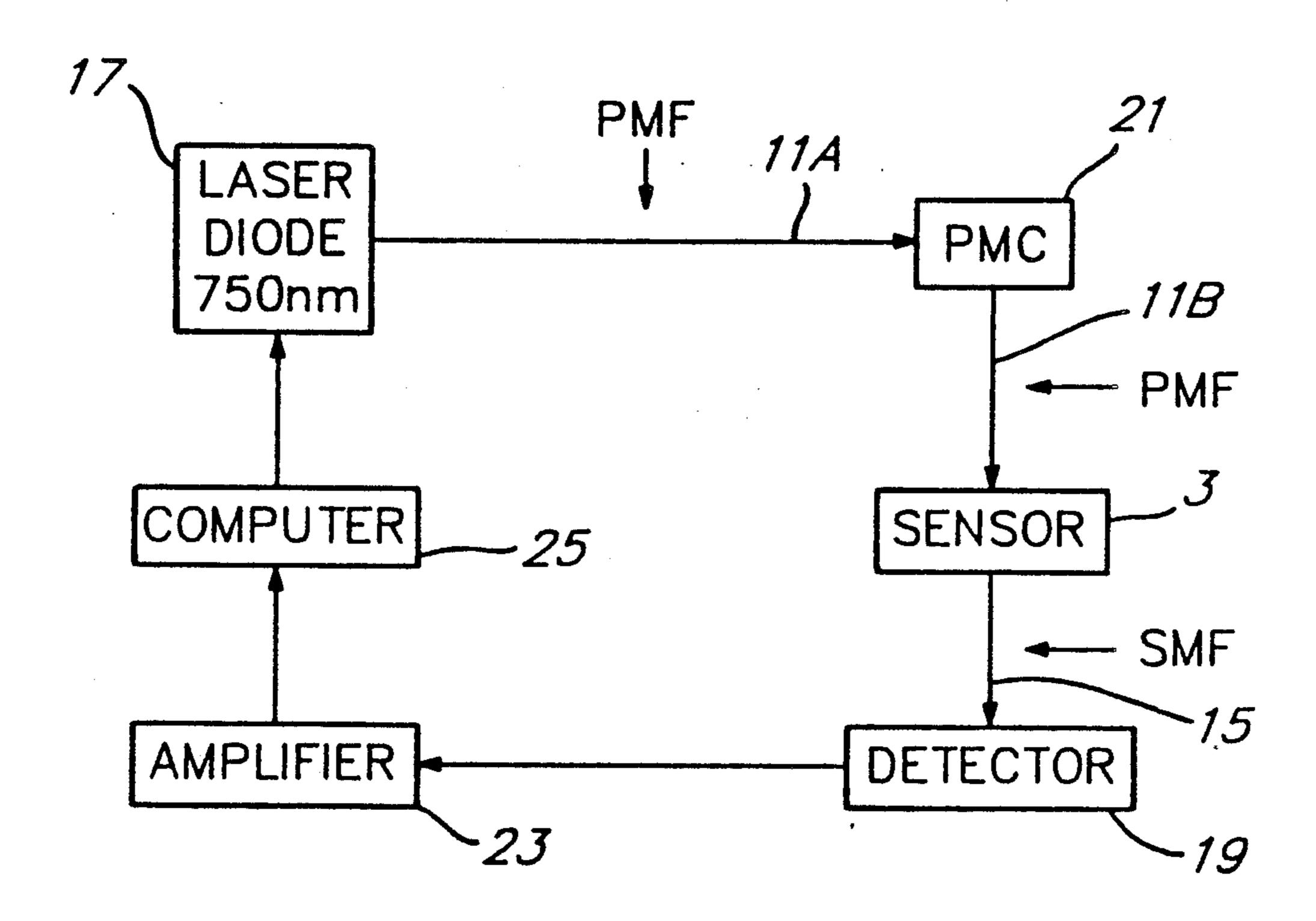
PMC - Polarization Maintaining Connector
