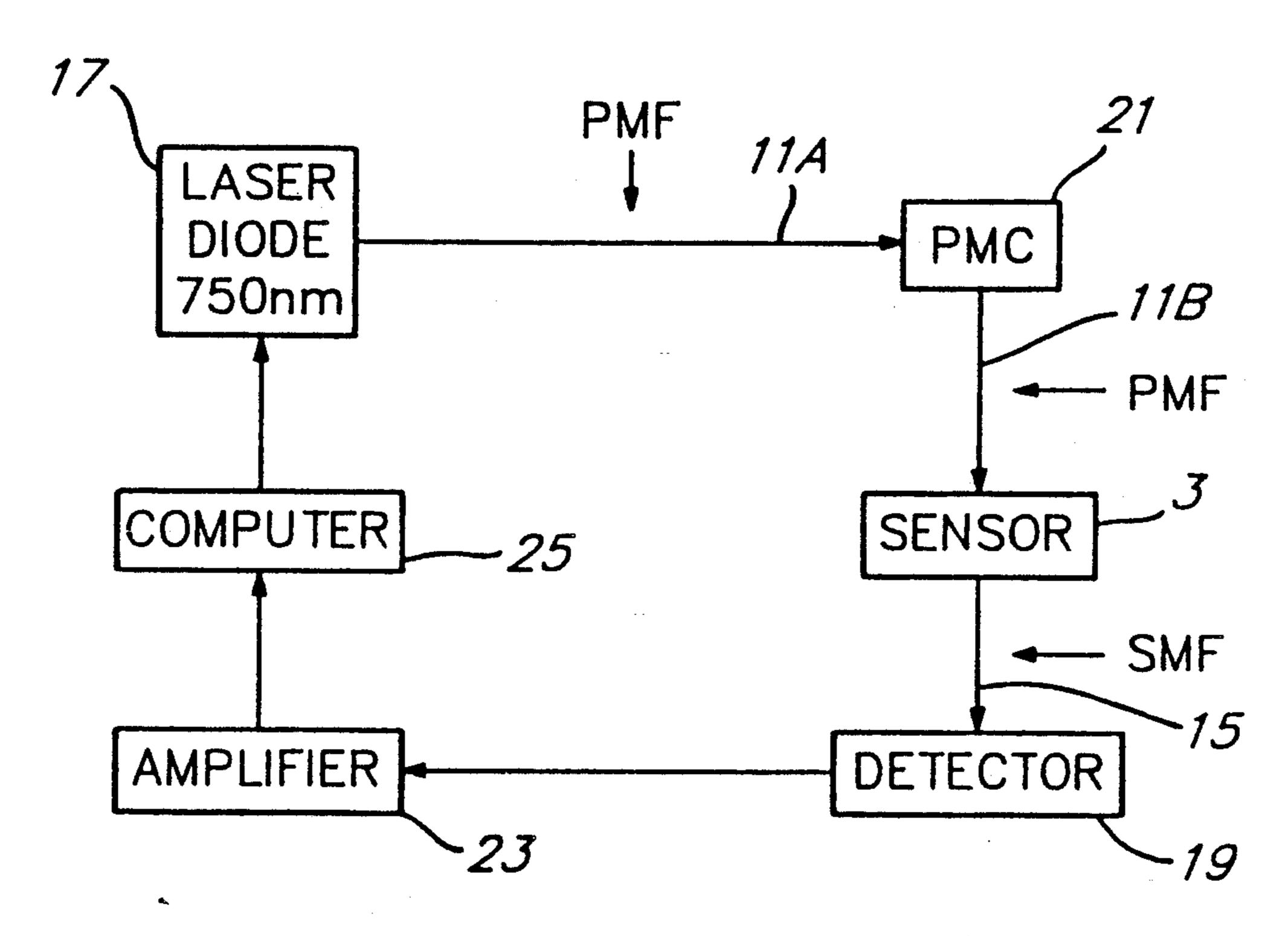
PMC - Polarization Maintaining Connector
