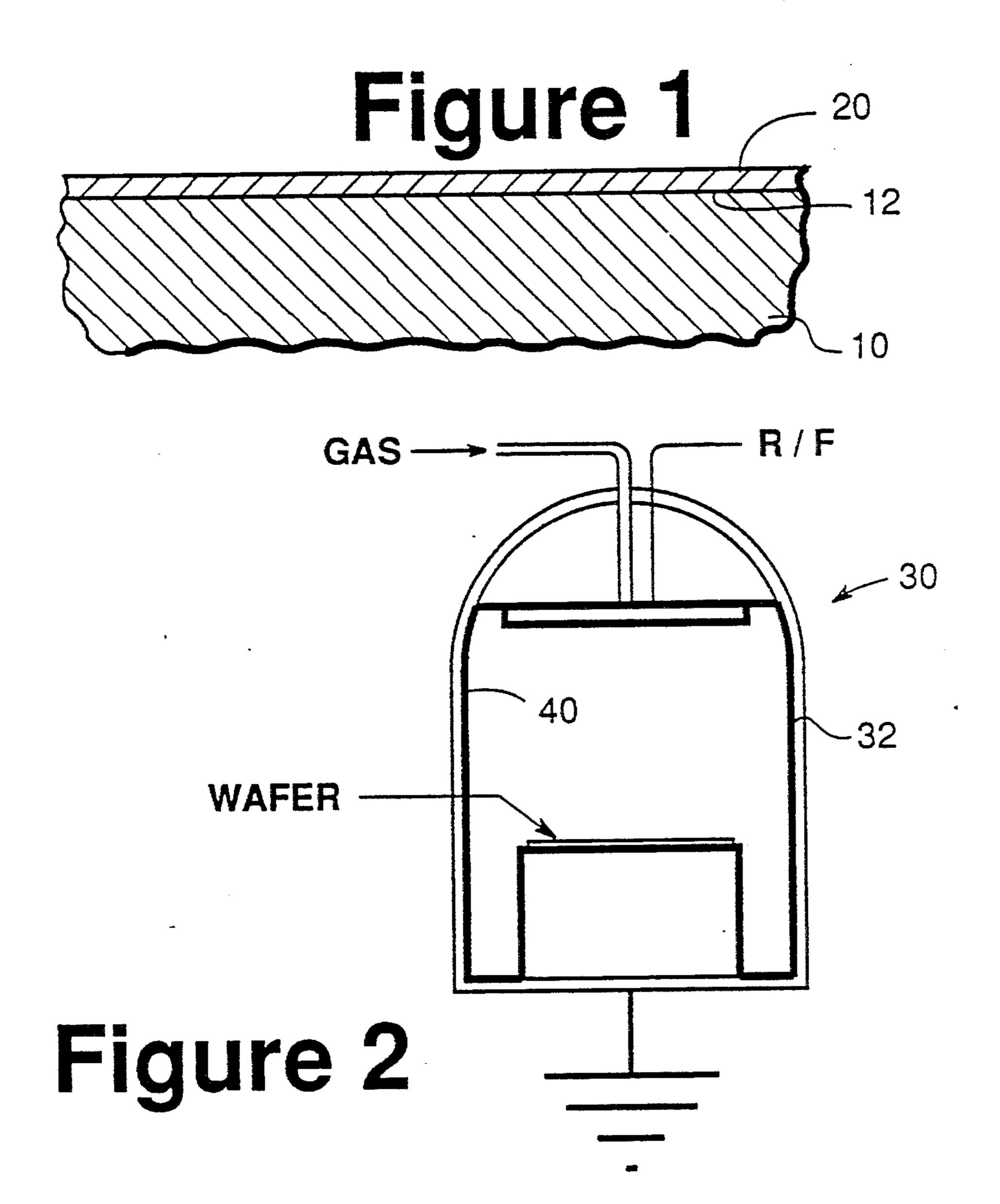
FORMING A HIGH PURITY ALUMINUM OXIDE FILM ON AN ALUMINUM SUBSTRATE SUCH AS THE INNER SURFACE OF AN ALUMINUM REACTOR USED FOR PROCESSING SEMICONDUCTOR WAFERS
