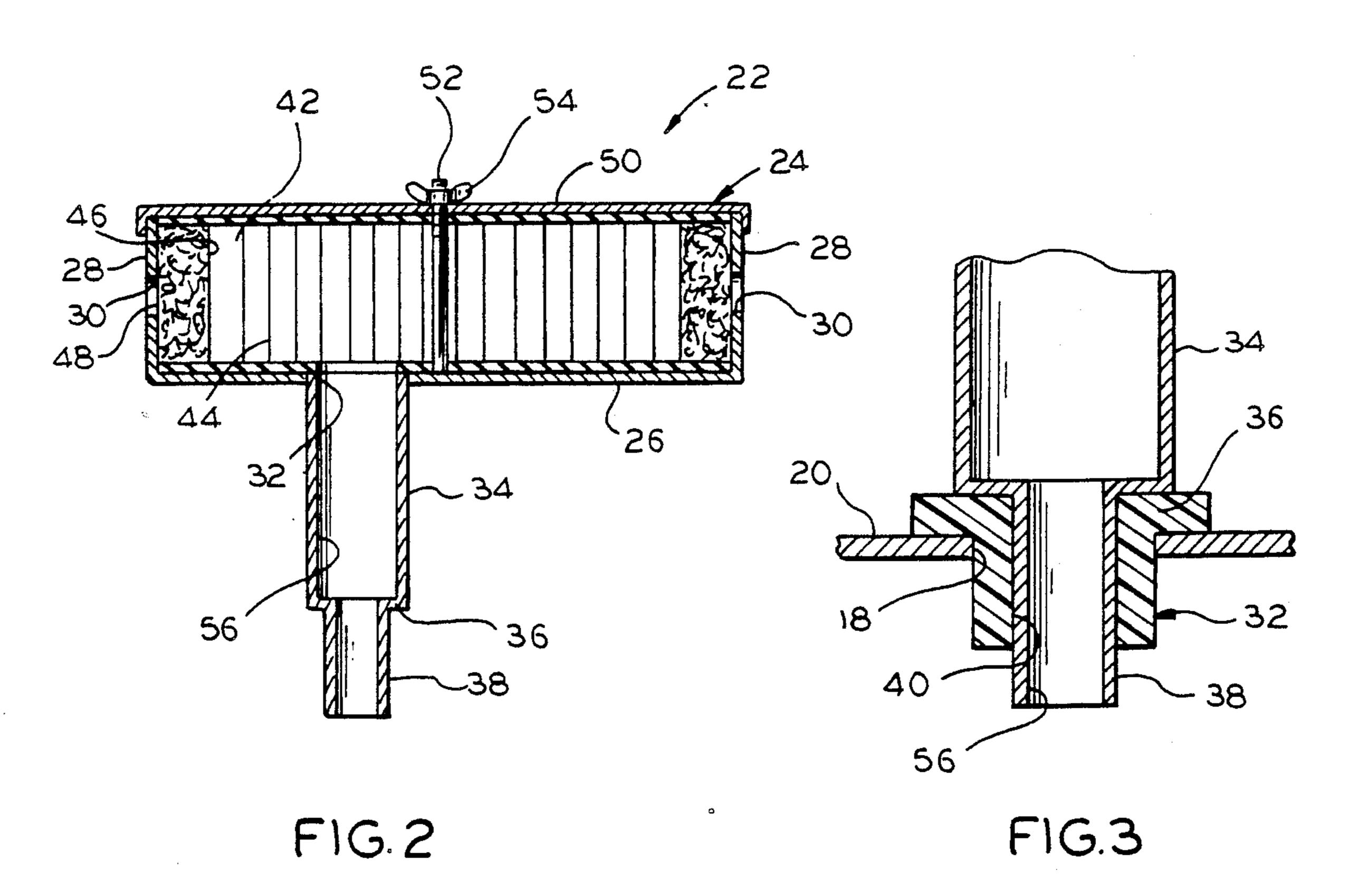
extends from the bottom wall communicates with the inlet and is slidably received in an exhaust outlet from
