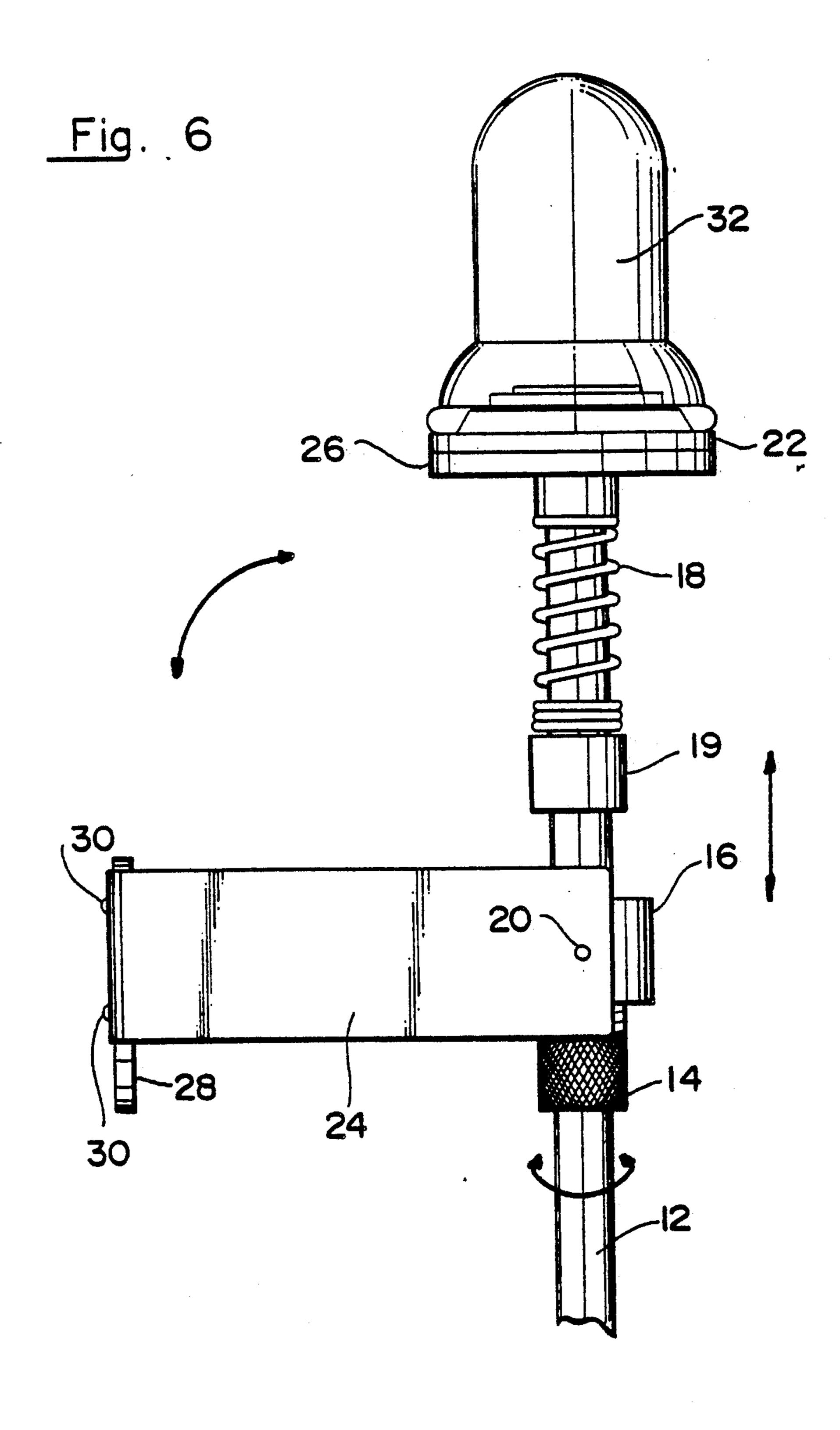
cate the three (3) degrees of freedom of movement of the clamping mechanism.
