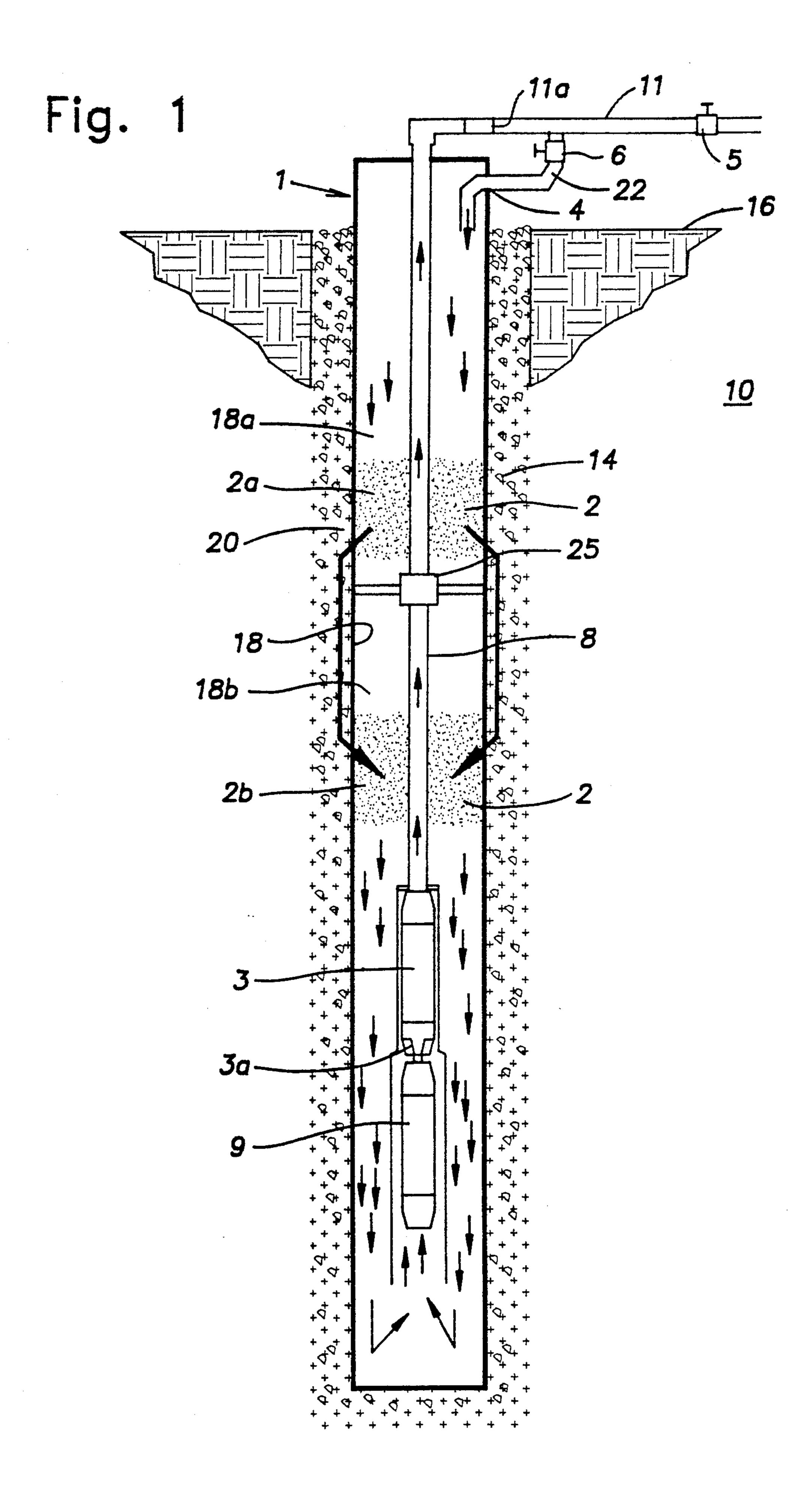
water containing at least one additive is recirculated through the well. The recycle flow is through an adja-
