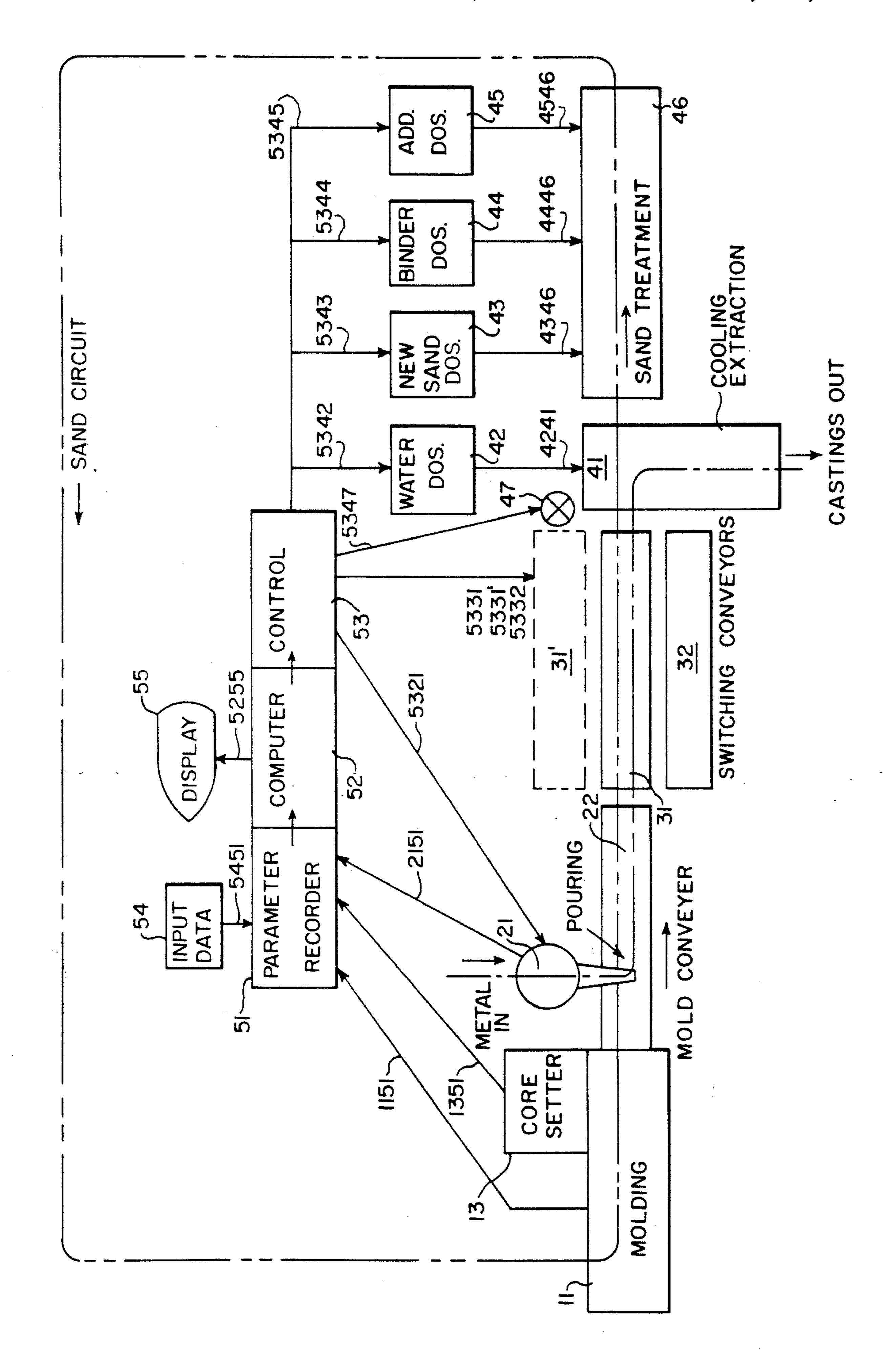
whereby it is also achieved that the various sensing and control functions can easily be changed by a simple reprogramming of the equipment.
