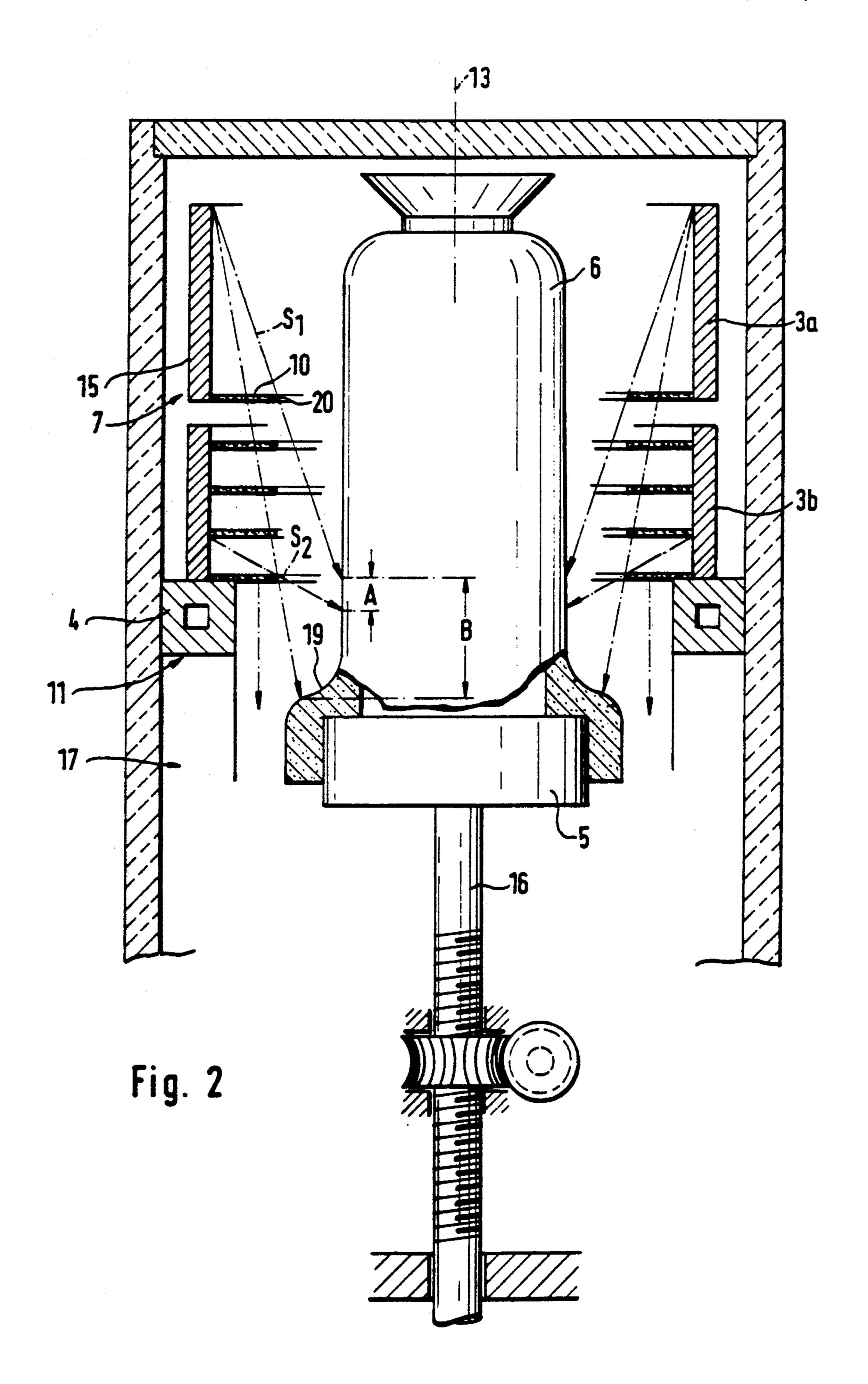
gap greatly constricts the radiation path and thus opposes any flattening out of the temperature gradient.
