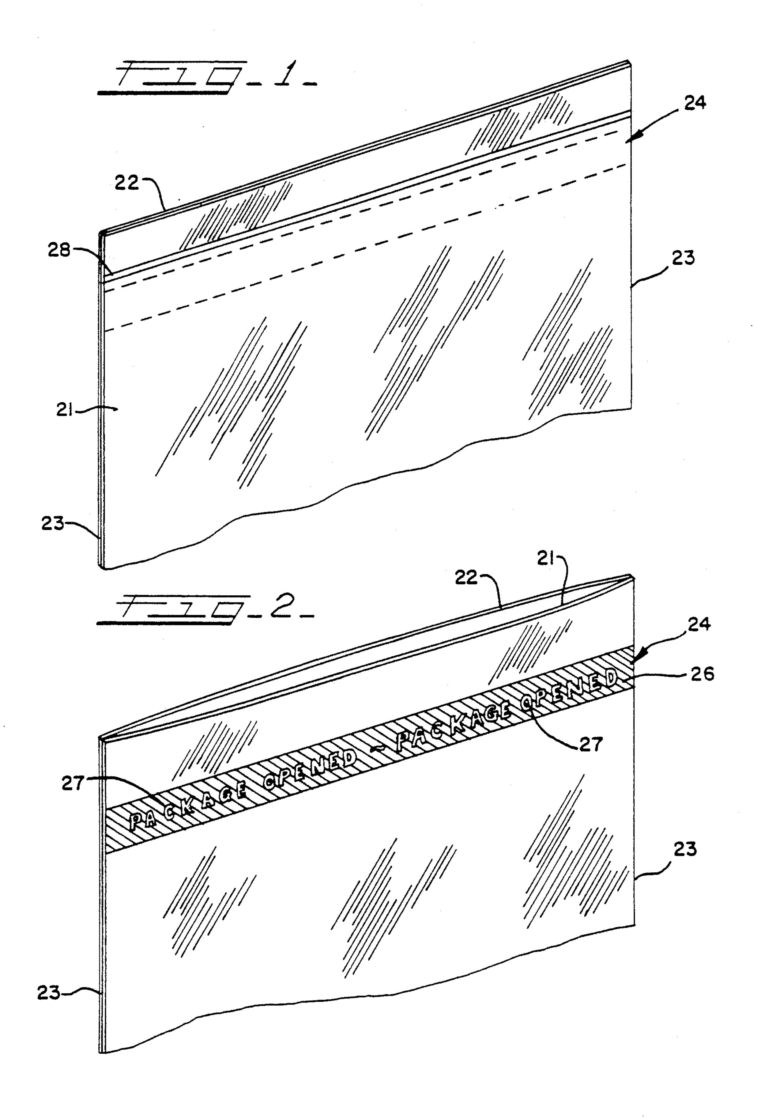
PACKAGE HAVING ENGRAVED LETTERING PEEL SEAL TAMPER-EVIDENCE MESSAGE
