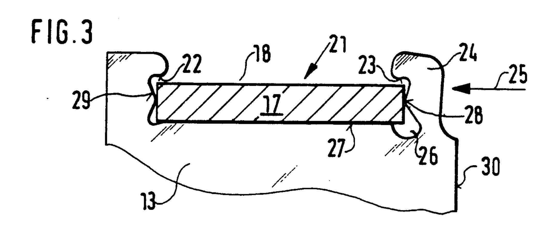
clamping of the armature in the recess in the closed position of the bendable projection.
