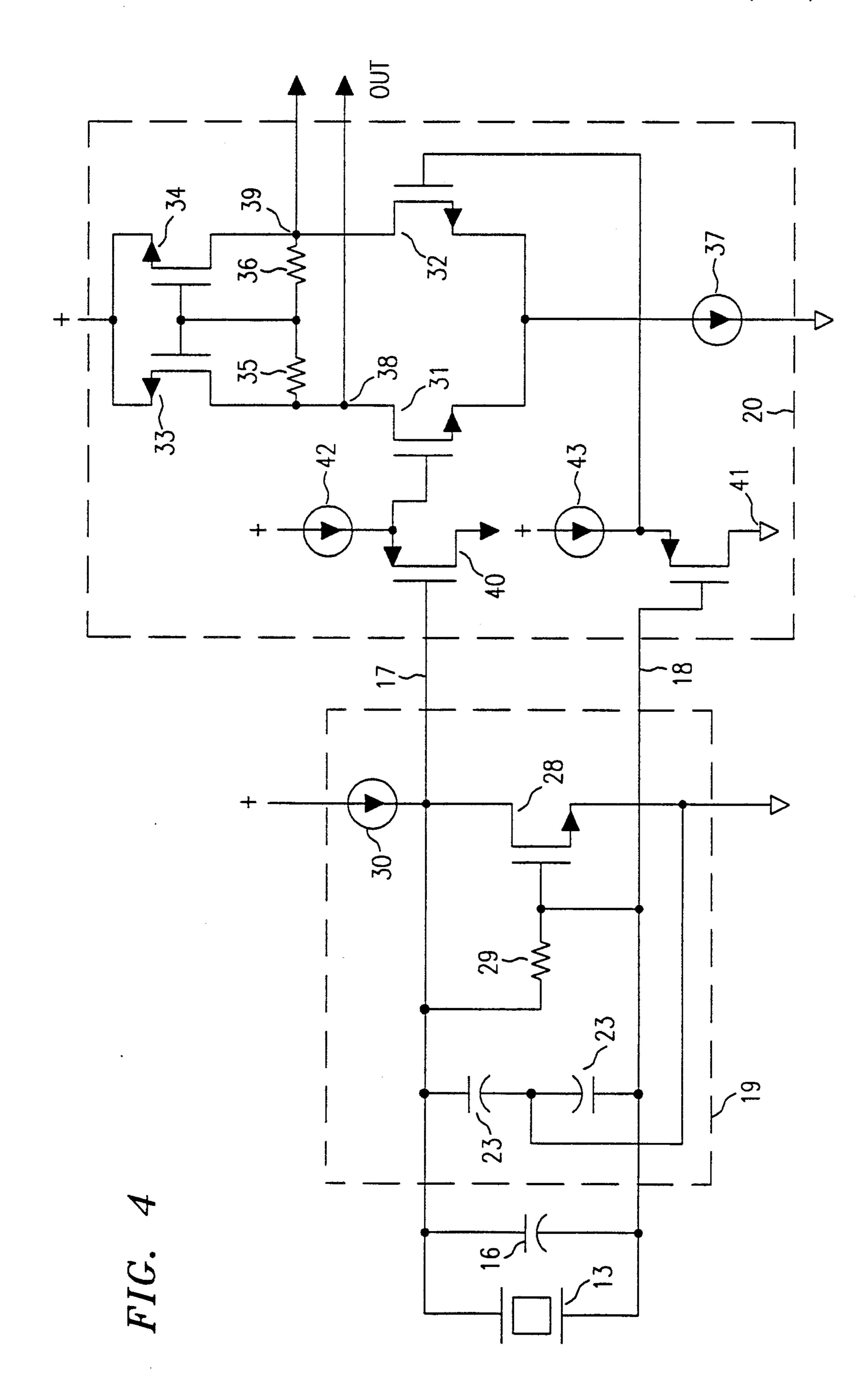
resonator used to determined the operating frequency of the oscillator.
