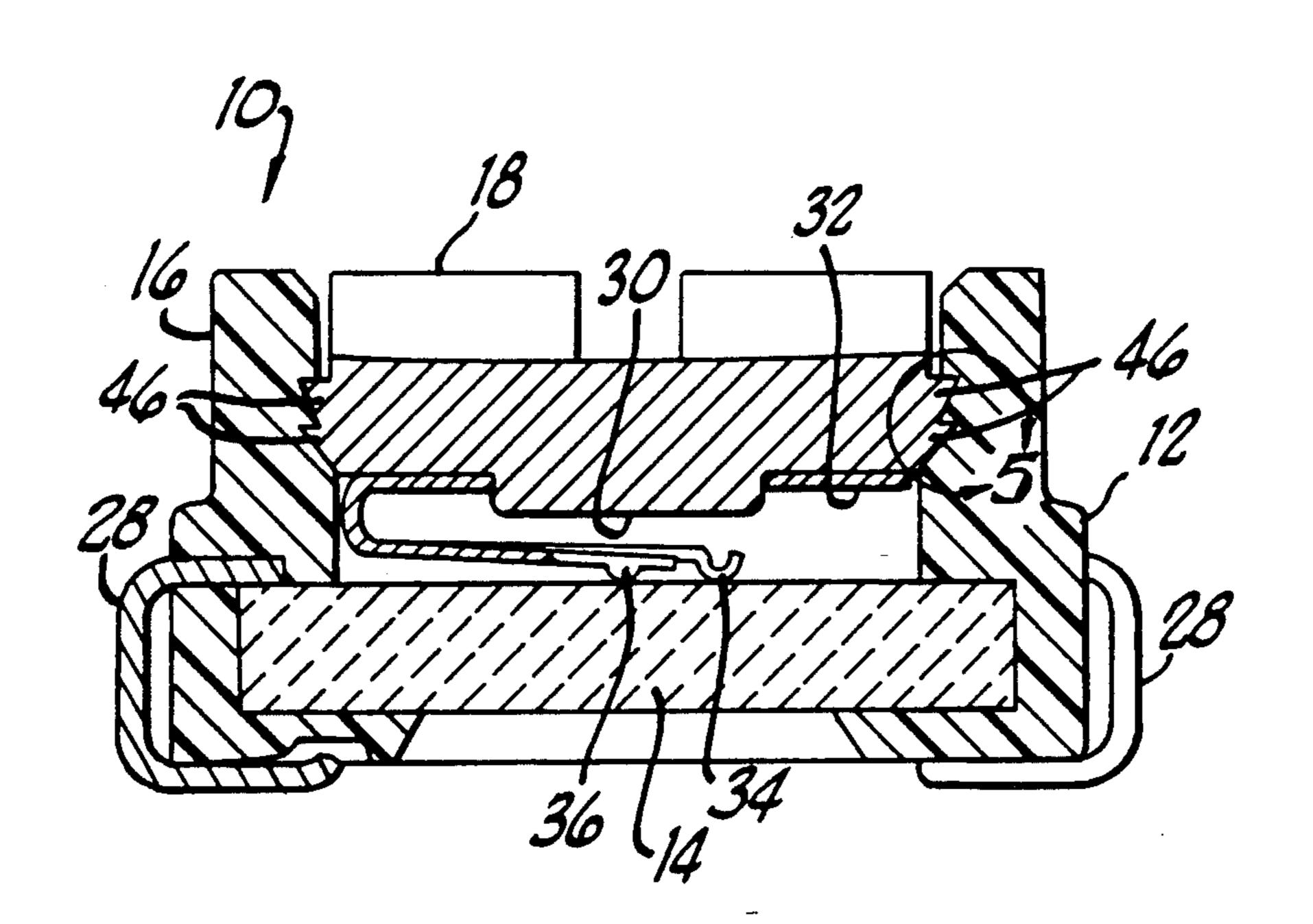
SINGLE TURN POTENTIOMETER WITH DIRECT ROTOR-TO-HOUSING SEAL
