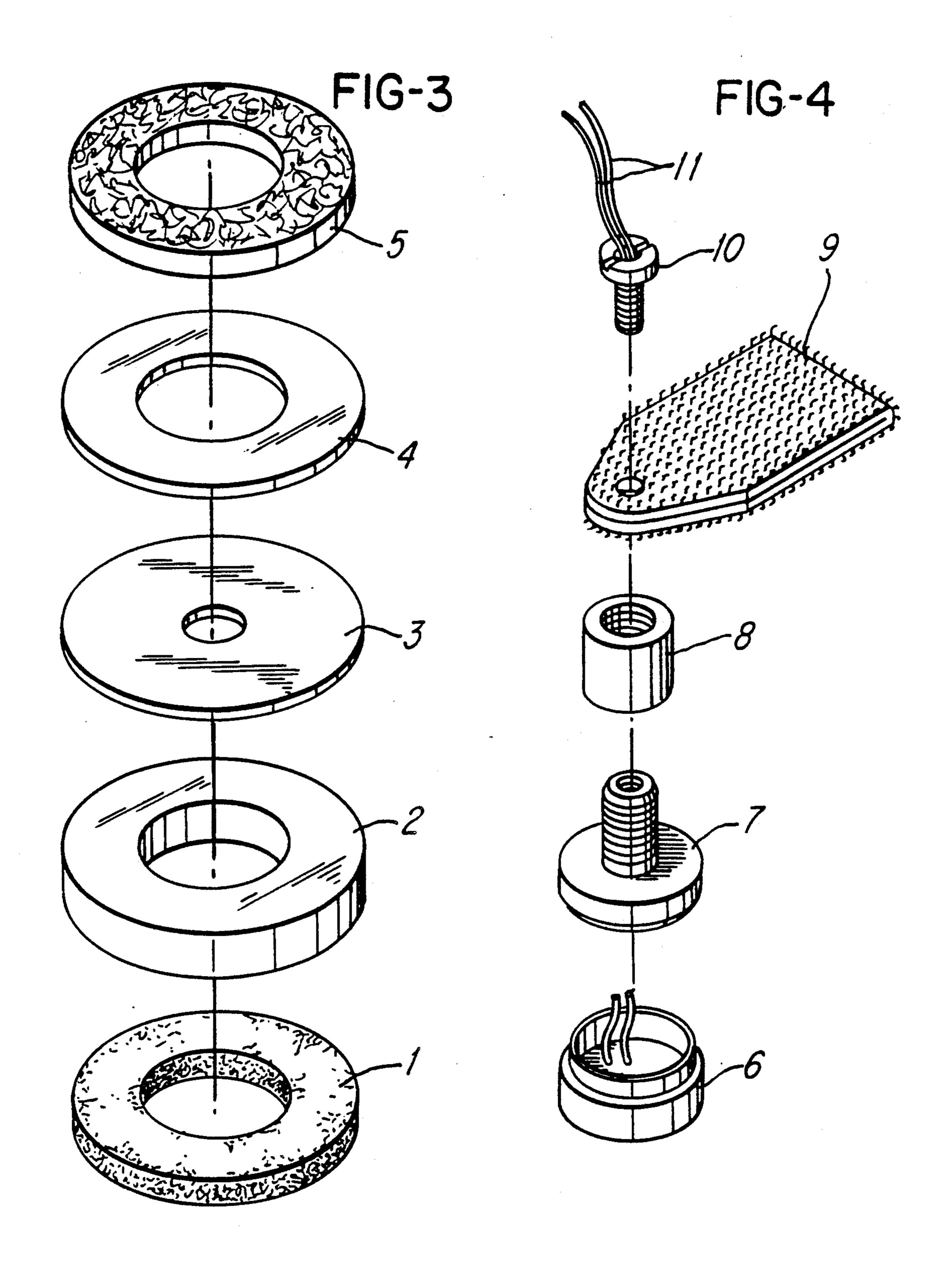
FIG. 4 is an exploded view of the transducer segment of FIG. 2.
