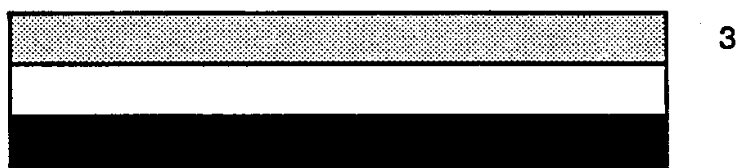
Fig. 6b. Positive photoresist is applied over the polyamic acid film and soft baked.
