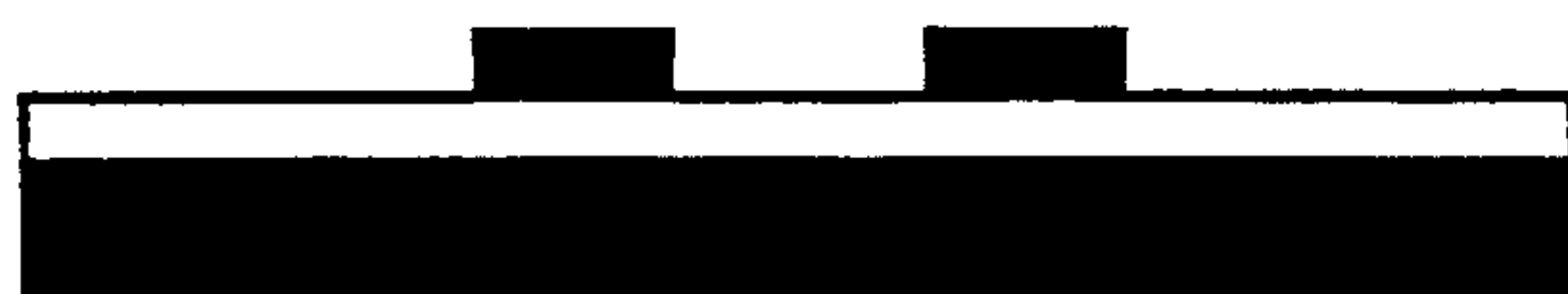
Fig. 4d. The photoresist is stripped away removing with it any overlying metal.
