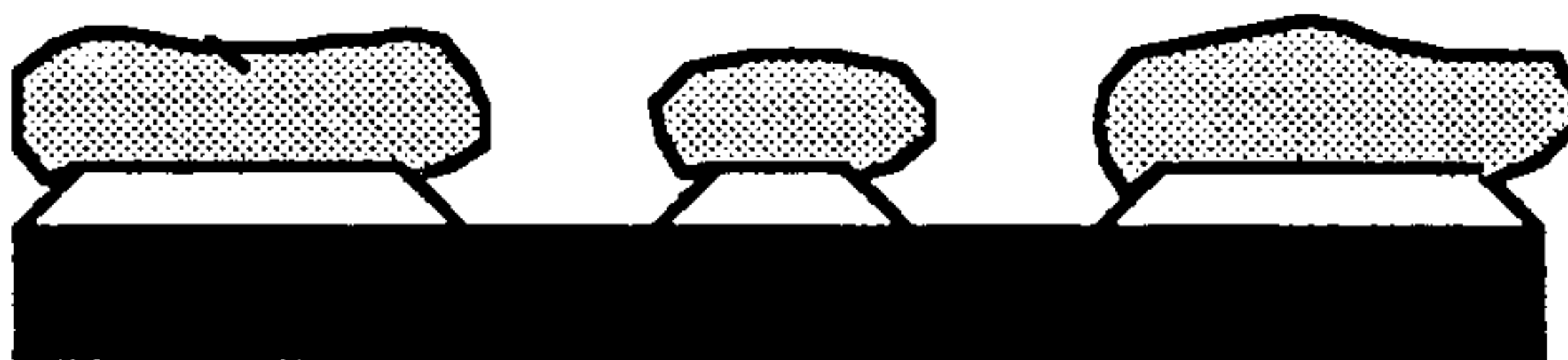
Fig. 8d. The structure is baked at temperatures >150^\circ causing photoresist deformation and converting the photoresist to a chemically intractable form.
