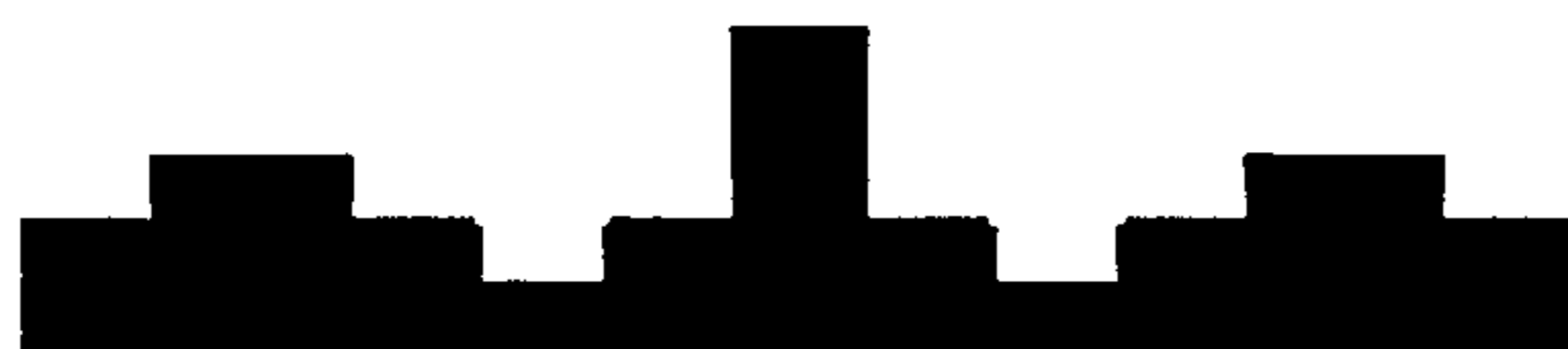
Fig. 11d. The masking structure is removed by dissolving the release layer in an alkaline medium.
