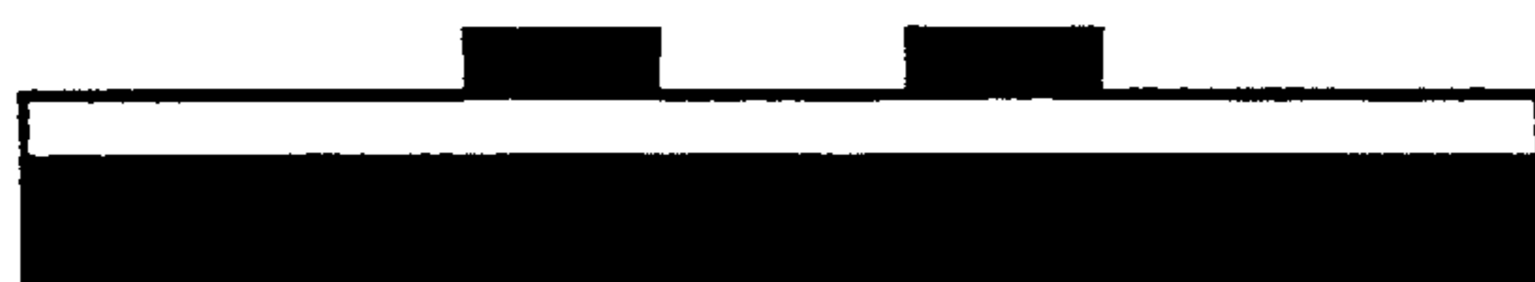
Fig. 4d. The photoresist is stripped away removing with it any overlying metal.
