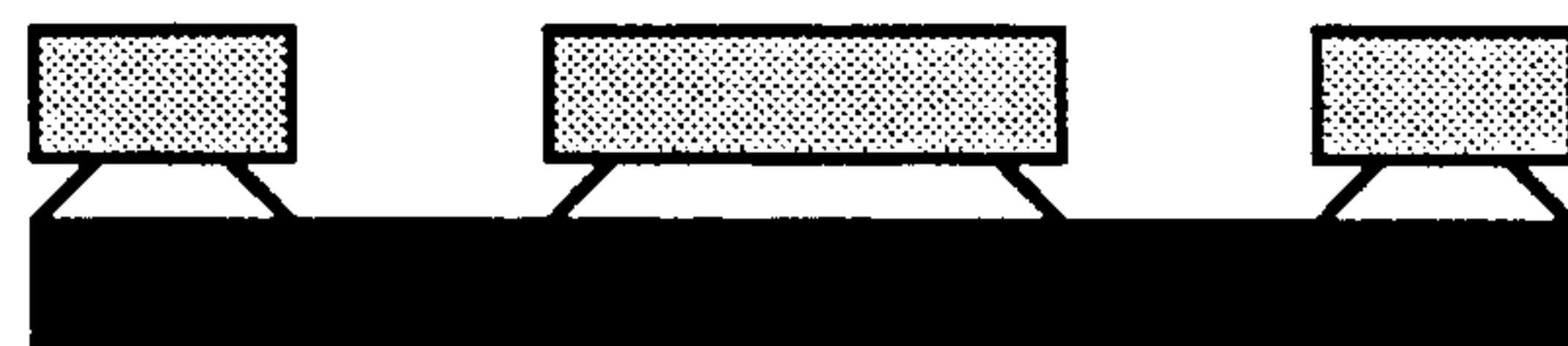
Fig. 5d. The photoresist and release layer are developed in dilute aqueous base, producing features with non-vertical walls in the release layer level.
